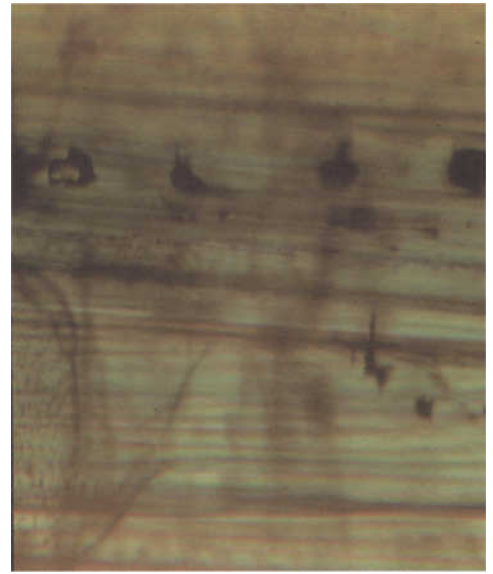
Figure 4: Growth and colour zoning approximately parallel to the basal pinacoid in I.G. Farbenindustrie synthetic emerald; some of the growth planes are not exactly parallel to each other. View perpendicular to the c-axis, immersion, 80x
