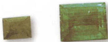
Figure 11: Chromium- and nickel-bearing I.G. Farbenindustrie synthetic emerald (left) and chromium-bearing Chatham synthetic emerald (right). The right-hand sample measures 9 x 7.3 mm (photo by H.A. Hänni)
