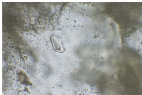
Figure 5b: Small idiomorphic albite crystals frequently occur in emeralds from Sandawana. The Raman spectrum of this crystal is shown in Figure 6 (feldspar II). Transmitted light, magnified 175x.
