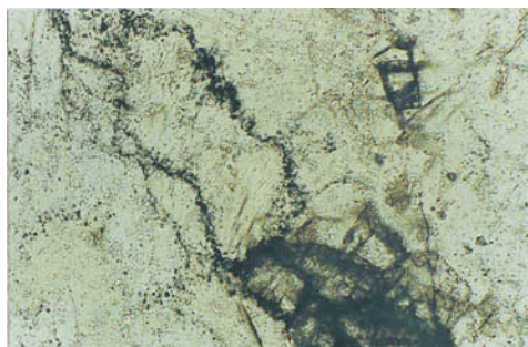
Figure 11: Black pigment concentrated along grain boundaries. Plane polarised light; field of view about 6 mm across.
