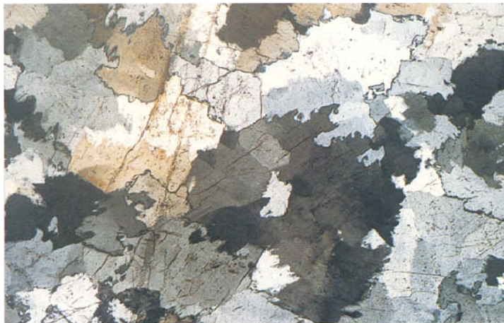
Figure 5: Granular interlocking texture of jadeite crystals; crossed nicols; field of view about 6 mm across.
