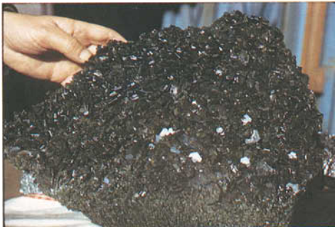
Figure 3: Synthetic moissanite produced by the Acheson process for abrasives use: (a) a typical black crystal cluster; (b) faceted yellow and green stones, the largest is 0.52 ct. Photos by K. Nassau.
