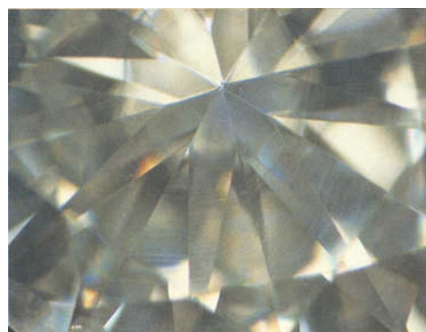
Figure 9: In diamond the polishing orientation must be repeatedly changed for successive facets because of its directional hardness; synthetic moissanite can be polished in a relatively consistent direction as is shown by the polishing lines on the facets of this stone, magnified 32x. Photo by Shane F. McClure, courtesy of GIA.
