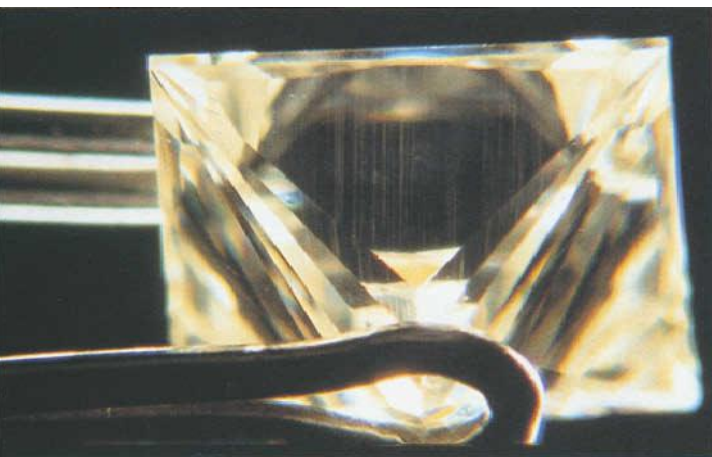
Figure 7: The most common inclusions in synthetic moissanite are thin white needles, generally parallel to the optic axis. Photo by Gary Roskin.
