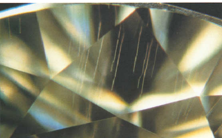
Figure 8: In a few synthetic moissanites offsetting bends occur in the needles. Photo by Gary Roskin.
