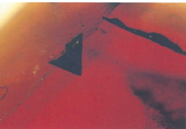
Figure 4: Black triangular crystal of ?hematite in synthetic alexandrite, \times 63 , oblique light (photo: I. Quintens).
