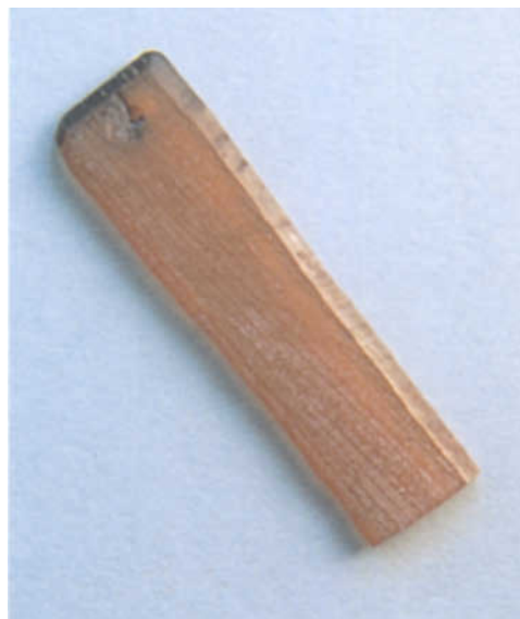
Figure 4: Crystal of hydrothermal yellow synthetic sapphire grown on a seed parallel to a prism b ( 10\bar{1}0 ); the absorption spectrum of the synthetic yellow sapphire is comparable to the spectrum of basaltic type natural sapphires coloured predominantly by iron. Size of sample about 35 x 10 mm; photo by M. Glas.
