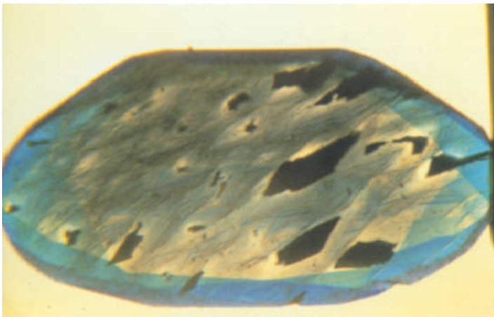
Figure 3: Boundaries of variable orientation between subindividuals and colour zoning in synthetic bluish-violet sapphire; large cavities with multiphase fillings appear opaque in this orientation of the sample. Immersion, magnified 30x.
