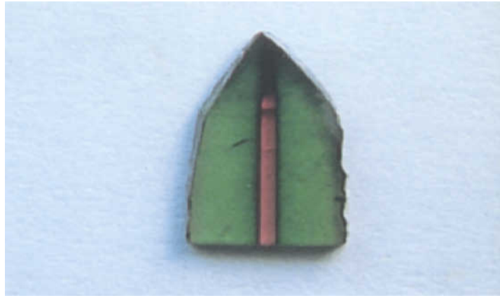
Figure 5: Plate of hydrothermal synthetic green sapphire grown on a seed parallel to a negative rhombohedron -r \{01\bar{1}1\} ; the absorption spectrum of the synthetic green sapphire reveals absorption bands of bi- and trivalent cobalt. Size of sample about 12 \times 8 mm; photo by M. Glas.
