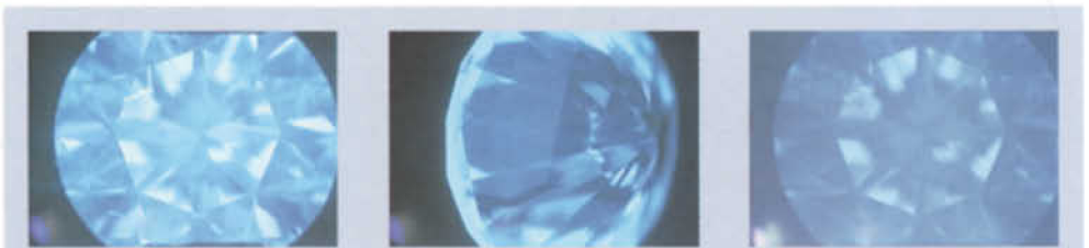
Figure 4d: De Beers white synthetic diamond, 0.60 ct (98–64). The characteristic internal structure of the synthetic origin of this stone is clearly evident. The last image records the strong and persistent phosphorescence. Stone 98–54 (0.24 ct) is similar.
