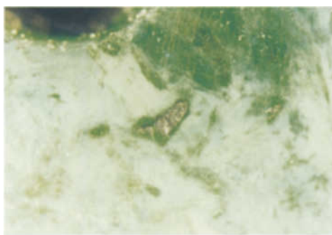
Figure 4: Detail of the back of the sample showing, as confirmed by EDS analyses, a relict grain of chromite (dark/metallic) surrounded by a deep green kosmochlor rim and an albite-rich matrix (the mineral association Chr+Kch is 1 mm long).
