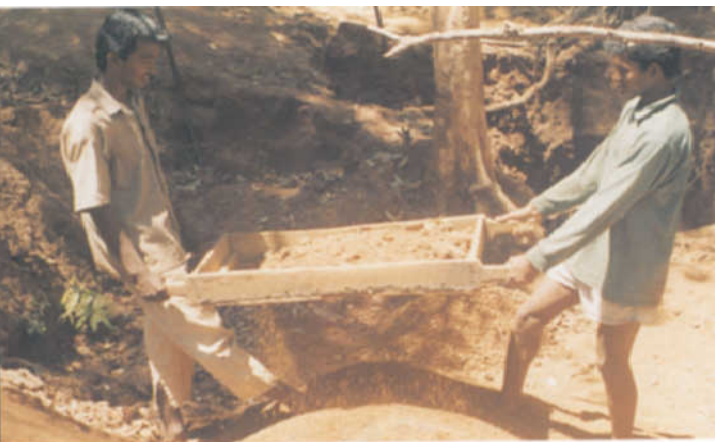
Figure 7: Gem-bearing sediments being sieved to remove the fine-grained fraction. This method is adopted when water is scarce in the dry season.
