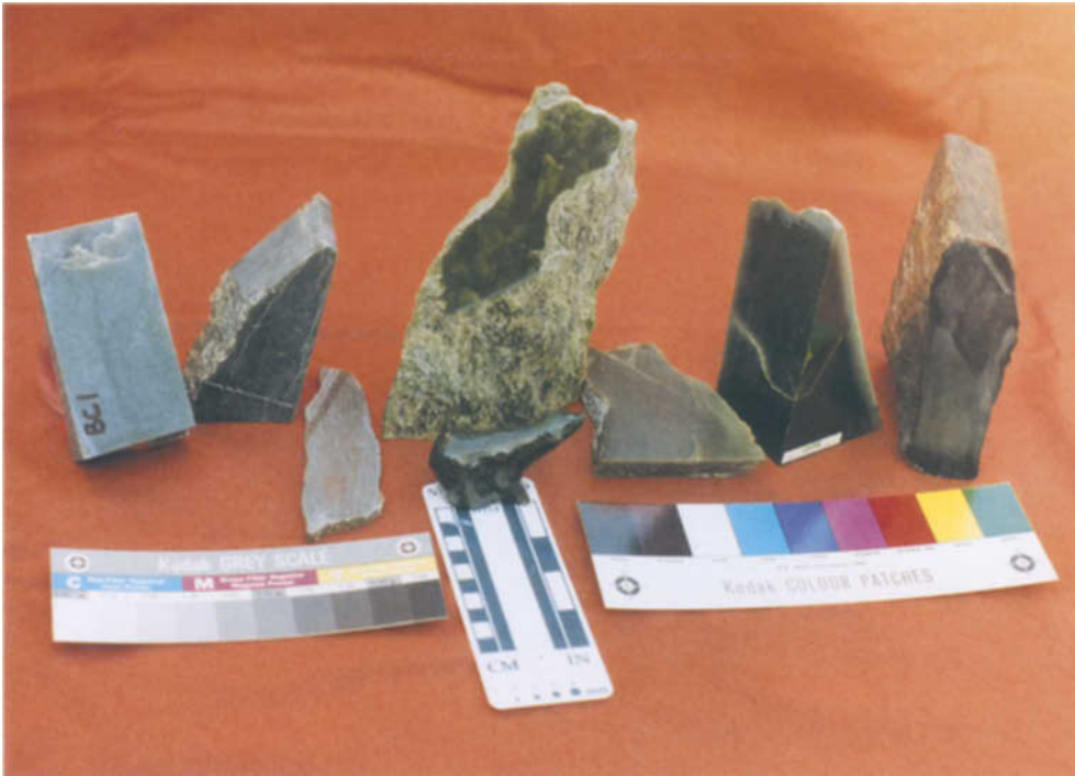
Figure 4: Suite of samples, from left to right, ortho-nephrite jade from Canada (BC1, 2, 3 and 4) and para-nephrite jade from Australia (SA1, 2 and 3).
