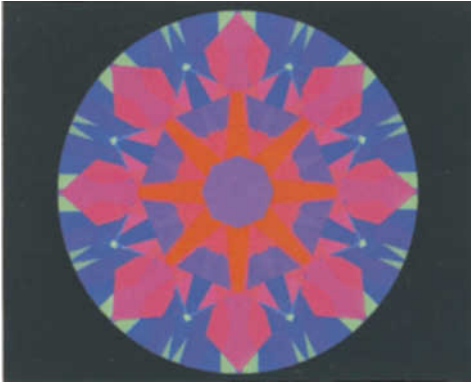
Figure 12: Reflection source detection of simulation of bottom diamond in Figure 11c with 32.6° crown angle.
