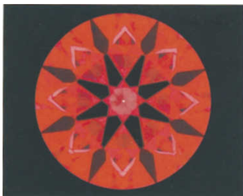
Figure 13: Firescope® image of 'Ideal' cut diamond with 34.5° crown angle (courtesy of Eightstar® Diamond Co.)
