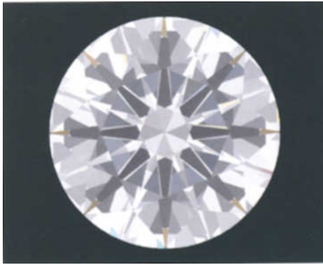
Figure 16: Parker's cut with a 55.9% table, 25.5° crown angle, and 40.9° pavilion angle.
