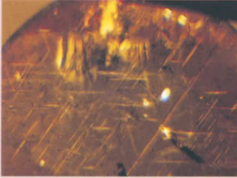
Figure 1: Three sets of birefringent lamellae that form an equilateral triangular pattern are observed in a view parallel to one of the three-fold axes of the host. Immersion, crossed polarizers, magnified 80x. Photomicrograph by K. Schmetzer.
