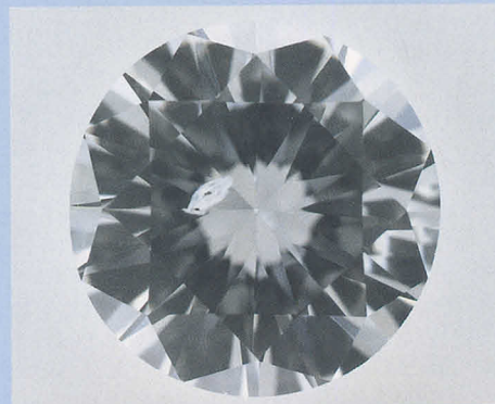
Figure 1b: After KM treatment. Black coloration has been removed from the inclusion. The size of the original inclusion area when viewed from the face-up position does not appear to be changed.
