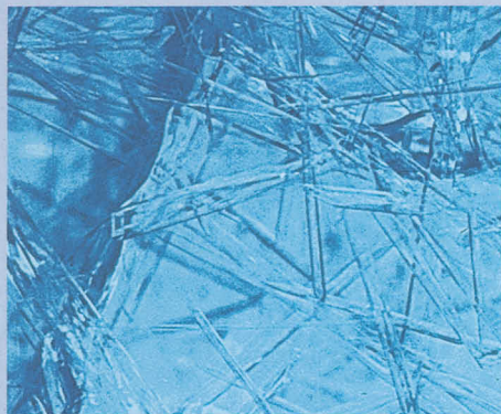
Figure 9: Sample A: Partially devitrified, and containing relatively coarse wollastonite crystals. Magnification approximately 15x. Photo by H.A. Hänni, SSEF.
