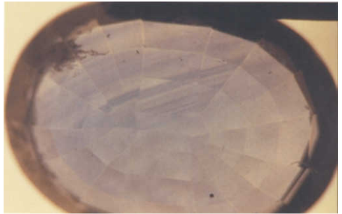
Figure 25: Pavilion view of the smaller surface-diffused corundum. The facet edges stand out as lighter in colour from the rest of the stone (diffused lighting conditions or immersion necessary). The parallel colour zoning is an internal feature related to the growth of the sapphire.
