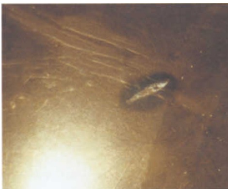
Figure 16: Silver concentrated in an imperfection on the surface of a stained cultured pearl.
