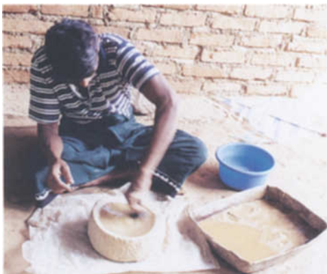
Figure 4: Grinding the lenses to get the right curvature in a special grinding stone selected from a series of such grinding stones with different curvatures.
