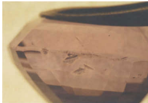
Figure 27: The larger surface-diffused corundum, which although being blue in daylight has a red hue on the microscope due to its chromium content. The pits below the girdle reveal that the diffusion process stops short of the pit edges but does diffuse into the bases of the pits themselves.
