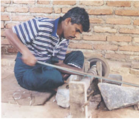
Figure 3: Grinding the quartz slice with a bow driven grinding wheel.
