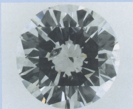
Figure 1a: Before KM treatment. Isolated black inclusion is located below the table of a brilliant-cut diamond (at 9 to 10 o'clock).
