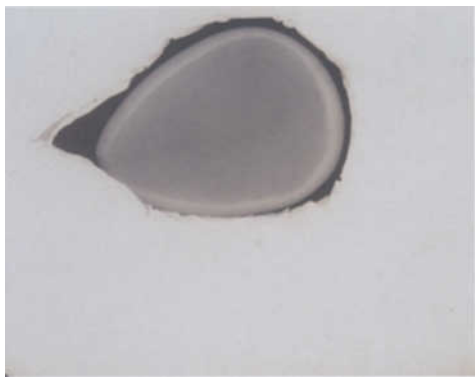
Figure 13: The radiograph of a drop-shaped natural hollow pearl filled with urea formaldehyde resin.
