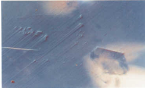
Figure 7: With observation using the differential interference microscope, it is apparent that the fracture on the right of the photograph existed before the cutting and polishing, and the laser-induced fracture on the left has been introduced after the polishing of the diamond.
