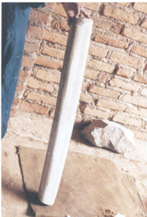
Figure 6: Wooden lap used for final polishing (made from Katu Erabadu).
