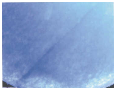
Figure 4: In dyed blue quartzite the colour is always concentrated on grain boundaries and along fractures. Length of the stone is 8 mm. Photo by S.T. Wu.
