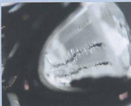
Figure 3: In both of these two KM-treated diamonds, the inclusion (which has the appearance of a centipede) leads to the surface of the table facet and has many smaller cleavages that protrude from its side. Black residue from the inclusion could not be removed completely by the treatment process and can be seen in areas along the laser-induced continuous fracture.
