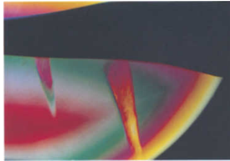
Figure 20: The wedge-shaped twinning seen in a synthetic amethyst observed on a microscope between crossed polars.
