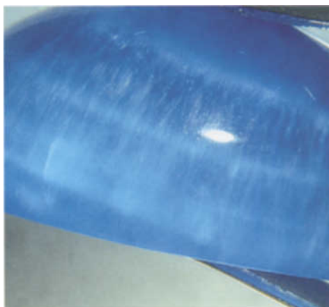
Figure 1: A 12.50 ct cabochon-cut glass imitation of blue chalcedony from Taiwan. The 17 mm long sample shows horizontal banding and perpendicular fibrous pattern. Photo by H.A. Hänni, SSEF.
