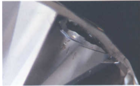
Figure 8: This boiled stone displays blue interference colour on the rim of the fracture.
