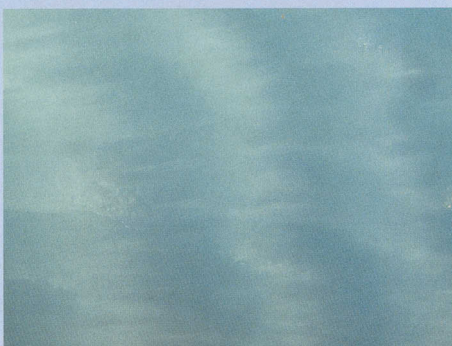
Figure 11: Sample C: Partially devitrified with very fine wollastonite crystals in a banding pattern. Magnification approximately 15x. Photo by H.A. Hänni, SSEF.
