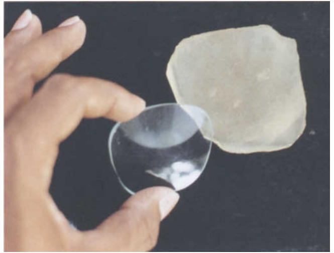
Figure 5: Bifocal lens (bifocal part constructed at the top owing to the limited capability of grinding implements used).
