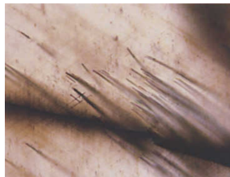
Figure 10: Dense network of rutile needles in an orientation parallel to two edges of the dodecahedron. Thin section, width of the sample about 0.45 mm.
