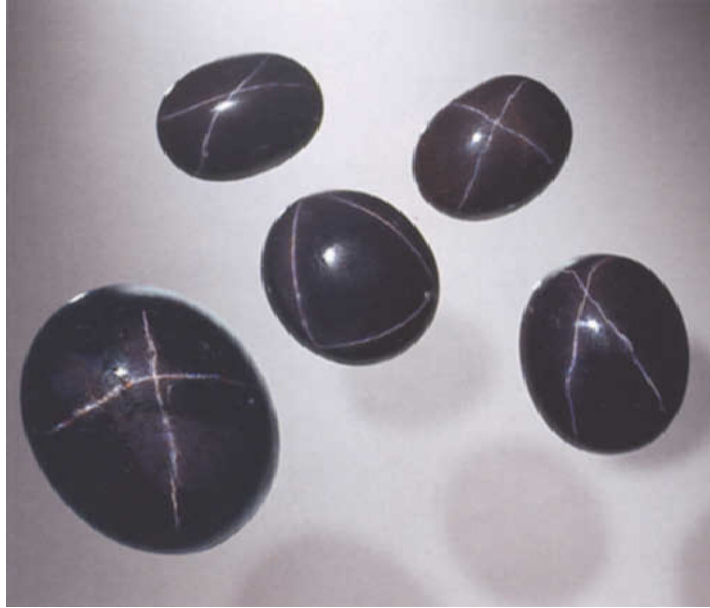
Figure 6: Asteriated garnet cabochons from Ambatondrazaka, Madagascar, revealing white four-rayed stars. The light bands of the four-rayed stars appear at different angles according to the orientation of the two-fold axis of the garnet in relation to base and dome of the cabochon. The cabochon in the centre is cut with a base perpendicular to a three-fold axis and shows the light bands of three four-rayed stars. Sizes of the samples are 19.5 x 15.4 mm to 11.1 x 8.9 mm, and weights vary from 34 ct to 5 ct. Photograph by M. Glas.
