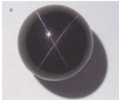
Figure 7: Garnet from Ambatondrazaka, Madagascar, cut as a complete sphere: a) In a view parallel to one of the two-fold axes a four-rayed star is observed. b) In a view parallel to one of the three-fold axes, the light bands of three four-rayed stars are observed. The diameter of the sphere is 13.0 mm, weight 18 ct. Photographs by M. Glas.
