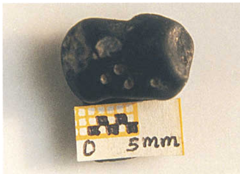
Figure 8: Several drill holes in a spinel as a result of testing the gauges of drill bits.
