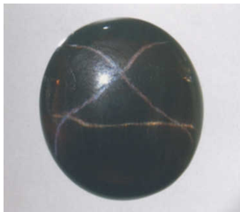
Figure 9: Asteriated garnet cabochon from Ambatondrazaka, Madagascar, revealing a white four-rayed star and a reddish-brown cat's-eye. It measures 19.2 x 17.2 mm, and weighs 33 ct. Photograph by M. Glas.
