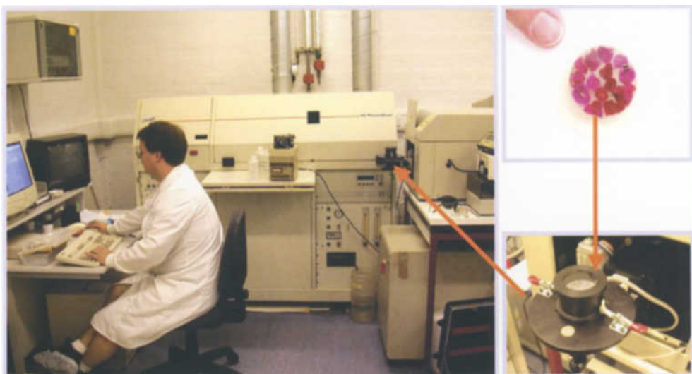
Figure 3: General view of the NERC Laser-ICP-MS system showing close-up views of the ablation chamber and a batch of Longido rubies prior to analysis.
