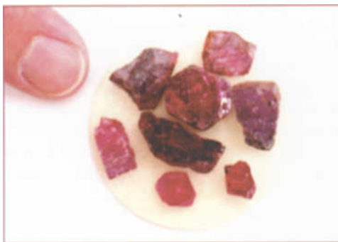
Figure 2: Uncut rubies from Chimwadzulu mounted on double-sided sellotape ready for introduction into the ablation chamber of the Laser ICP-MS system.
