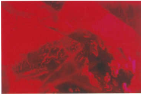
Figure 5: Some 'fingerprints' found with a glassy dark red substance (healing flux?), in the 2.60 ct Verneuil ruby (dark field illumination 35x).
