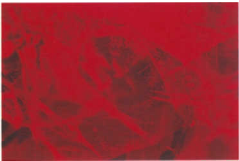
Figure 3: Numerous twisted wispy veil-like 'fingerprints' in the 2.60 ct Verneuil ruby, similar to those present in some Mong-Hsu (Myanmar) rubies (dark field illumination 30×).
