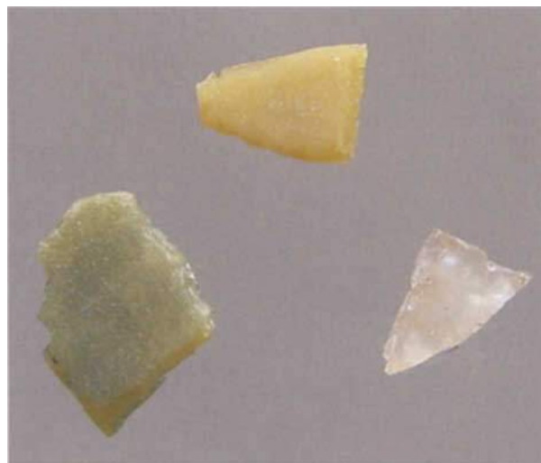
Figure 4: Light yellow, orange and green grossular. The orange and green colours were obtained after diffusion treatment of the light yellow material with Fe and Co, respectively. The stones have a diameter of about 8 mm.
