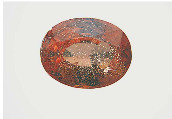
Figure 2a: Diffusion-treated originally pink or purplish-pink sapphire of 1.44 ct originating from Ilakaka, Madagascar; this sample was labelled 'deep diffusion treated' in Thailand. Photo by M. Glas.
