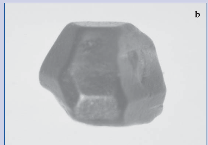
Figure 4: (a) Idealized drawing of the 2.35 ct greyish purple taaffeite crystal (clinographic projection); the sample exhibits two basal pedions (0001) and (000\bar{1}) [below, not visible] as well as three different hexagonal pyramids \{11\bar{2}3\} , \{11\bar{2}2\} , \{11\bar{2}\bar{2}\} and one hexagonal prism \{10\bar{1}0\} as crystal forms; (b) photo with the sample in the same orientation. Photo: K. Schmetzer.
