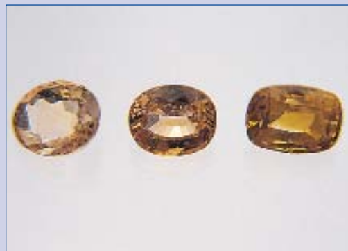
Figure 1b: Different types of orange or reddish-orange sapphires from Sri Lanka; untreated chromium-bearing sample (left), heat-treated chromium-bearing sample (centre) and heat-treated chromium-free sample (right); range of samples from 1.45 to 2.17 ct. Photo by M. Glas.
