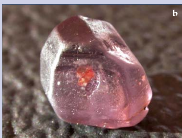
Figure 1a, b: This crystal of 2.35 ct and measuring 6.8 x 7.2 x 5.8 mm, is taaffeite with a bipyramidal habit and two opposing basal pedions; it is slightly waterworn. Photos: M. Burford.
