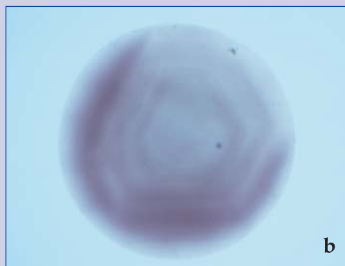
Figure 3: Even in immersion, the colour zoning of untreated Songea rubies and sapphires (a) may closely resemble the pattern observed for diffusion-treated material (b) from the same locality; sample (a) 0.54 ct, sample (b) 0.75 ct. Photos by K. Schmetzer.
