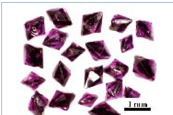
Figure 1: Ruby crystals grown from \text{MoO}_3 flux.
