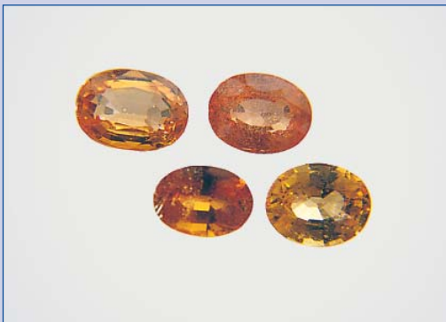
Figure 1d: Beryllium-diffusion-treated sapphires from Ilakaka, Madagascar; range of samples from 1.10 to 1.47 ct. Photo by M. Glas.
