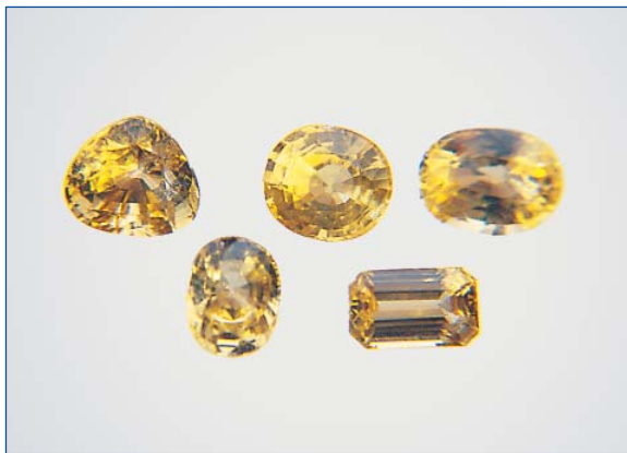
Figure 19: Beryllium-diffusion-treated, chromium-free yellow and yellowish-orange sapphires from Sri Lanka, range of samples from 1.17 to 2.15 ct. Photo by M. Glas.
