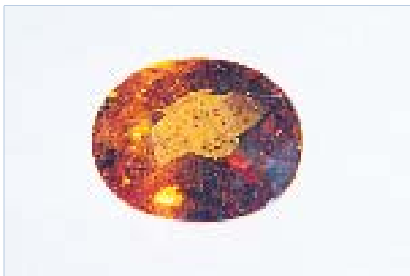
Figure 2c: Diffusion-treated originally pink or purplish-pink sapphire of 1.29 ct originating from Ilakaka, Madagascar. Photo by M. Glas.
