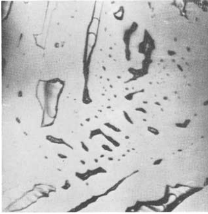
FIG. 45. Characteristic inclusions in topaz consisting of cavities filled with non-miscible liquids. 100 x
