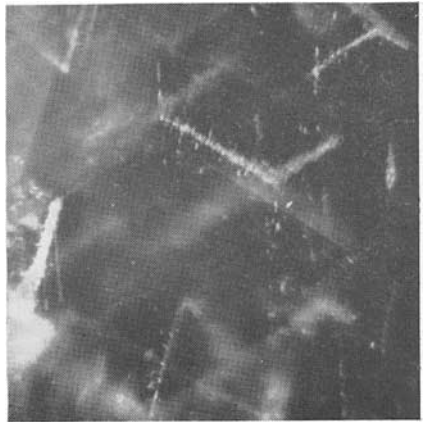
FIG. 40. Angular markings, which are characteristic of green metamict zircons from Ceylon. 300 x
