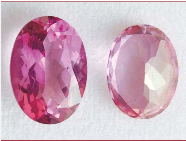
Figure 5: These two pink topazes are dye-coated on the pavilion facets of the samples. Different colour intensities are observed when viewed through the colourless crown and through the dyed pavilion. The stones are 18.0 × 13.0 mm and 15.8 × 12.0 mm, weights 15.17 and 10.59 ct. Photo by M. Glas.
