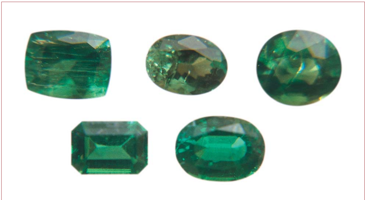
Figure 17: Different types of hydrothermally-grown synthetic emeralds; upper line left: Biron (Australia) synthetic emerald coloured by chromium and vanadium (1.49 ct, 7.9 × 6.4 mm), centre: Russian synthetic emerald coloured by chromium (grown in an autoclave with noble metal liner), right: Russian synthetic emerald coloured by chromium, iron, copper, and nickel (grown in an autoclave without noble metal liner); lower line: two samples of the new type grown by Tairus coloured by vanadium and copper. Photo by M. Glas.
