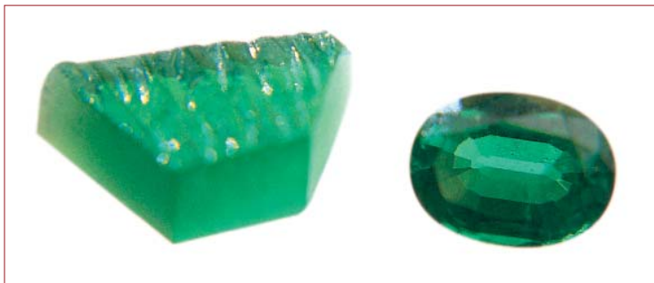
Figure 6: Faceted and rough samples of the new type of Tairus hydrothermally-grown synthetic emerald coloured by vanadium and copper; rough crystal plate of 3.23 ct ( 12.7 \times 6.6 mm), faceted stone of 1.16 ct ( 6.1 \times 8.1 mm). Photo by M. Glas.
