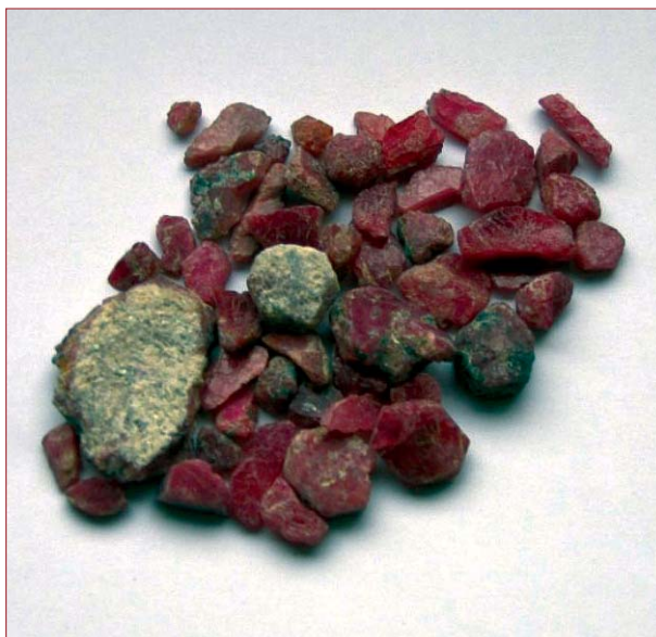
Figure 2: Ruby crystals from Madagascar with a saturated colour and numerous cracks. Their appearance can be significantly improved with a high RI glass.
