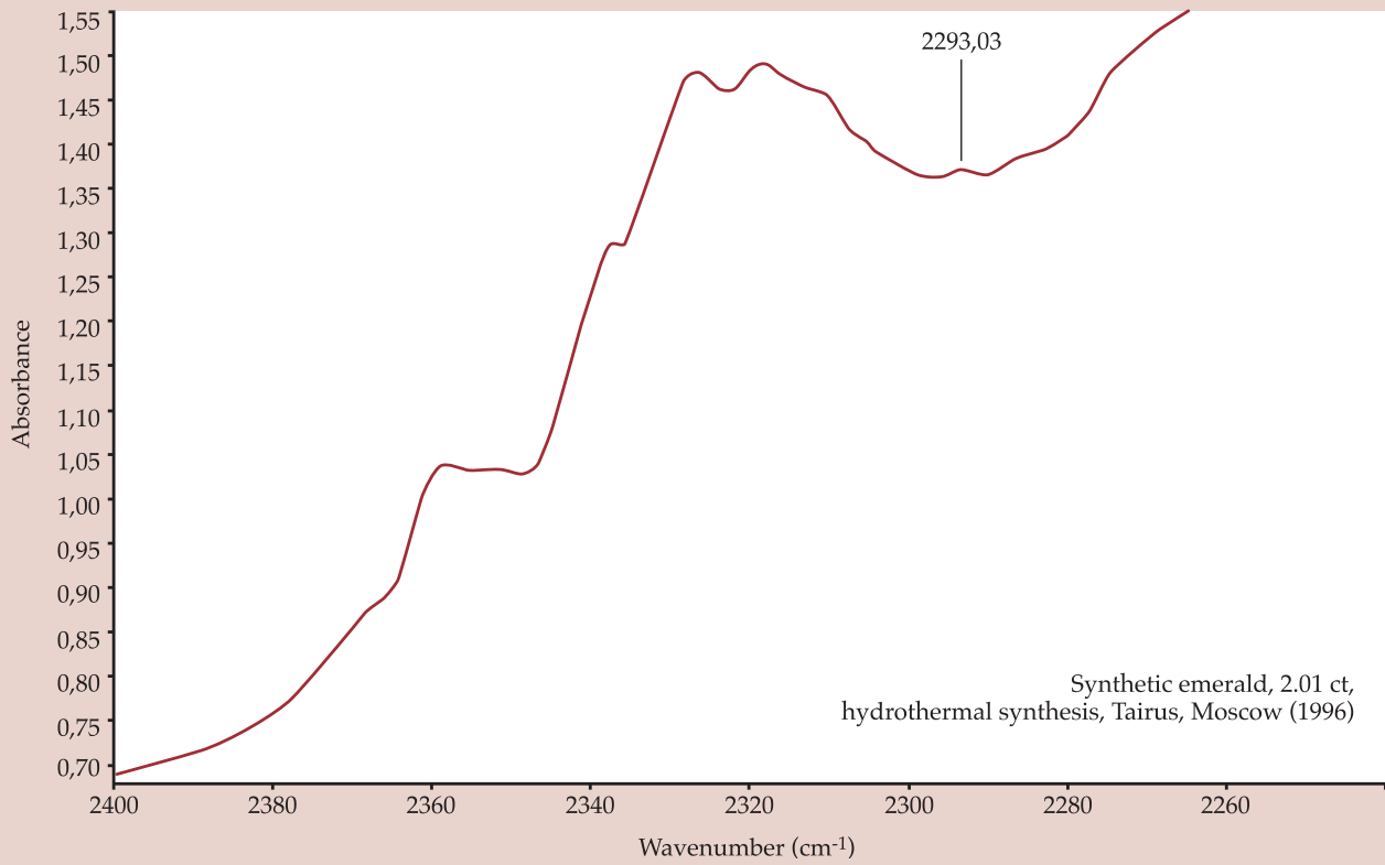
Figure 10a: The 2.01 ct synthetic Russian Tairus hydrothermal emerald exhibiting a 2293 cm -1 absorption band which is also present in natural emeralds.
