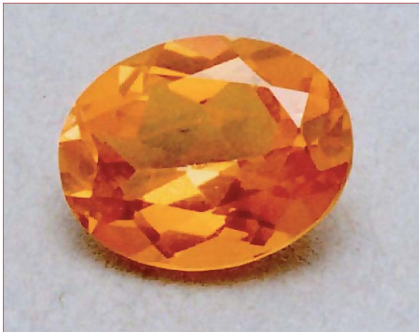
Figure 1: This surface-coated topaz is coloured by a thin iron-bearing layer on the pavilion of the stone; similar stones have been offered to gem dealers in Nigeria as natural topaz. The stone measures 10.1 × 8.0 mm, weight 2.95 ct. Photo by M. Krzemnicki, SSEF, Basel.
