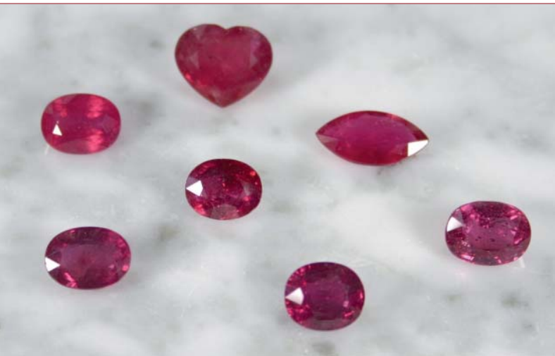
Figure 1: Faceted rubies from Madagascar with lead glass fracture fillings (weight between 4.03 and 12.58 ct).
