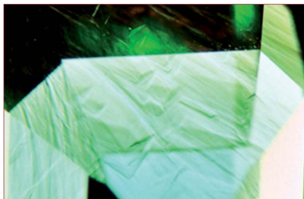
Figure 4: Characteristic chevron pattern is clearly visible in the 2.01 ct emerald cut hydrothermal Russian synthetic emerald (dark-field illumination 25x).
