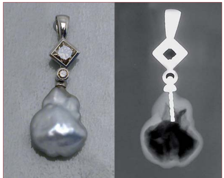
Figure 1: Beadless cultured Tahiti pearl – a so-called keshi – mounted as a pendant, with its radiograph showing a large irregular cavity (dark area). Length of the pearl 22 mm. Photo © H.A.Hänni, SSEF.
