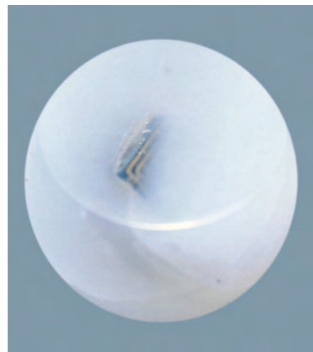
Figure 5: A composite shell bead that has been sliced and polished to show a small RFID chip (3 mm long) embedded within it. The information on such a chip can be accessed using an RFID reader. Photo by H. A. Hänni.
