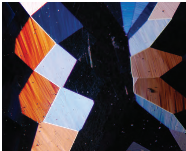
Figure 32: Swirl marks were evident in the glass (particularly on the left) when viewed with magnification and transmitted light. Polishing marks are also seen on some pavilion facets. Photomicrograph by Tay Thye Sun; magnified 15 \times .
