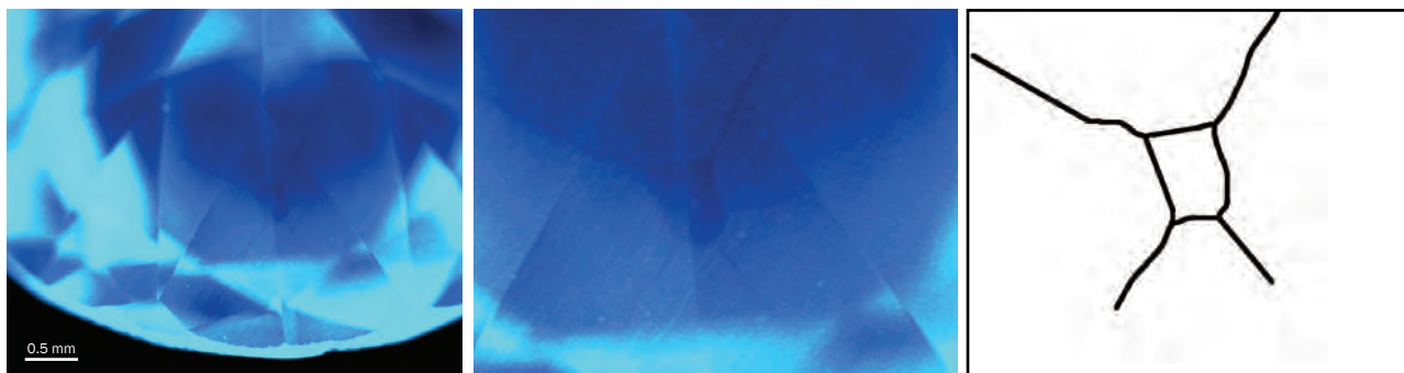
Figure 27: The DiamondView images of the 1.01 ct diamond show a luminescence pattern reminiscent of near-colourless HPHT synthetics, with a square core and four branches radiating from the corners. Photomicrographs and drawing by A. Delaunay.
