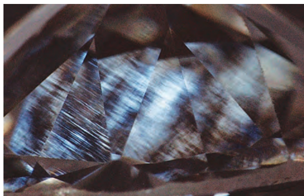
Figure 26: Banded graining is observed in the diamond between crossed polarizers. Photomicrograph by A. Delaunay; magnified 70×.
