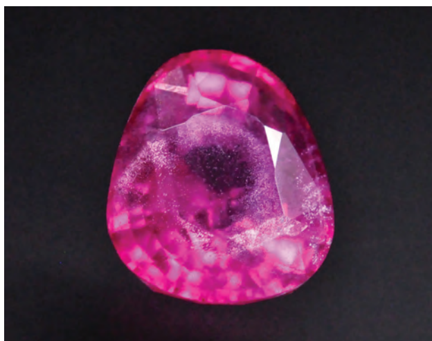
Figure 33: This 4.78 ct doublet, composed of synthetic ruby pieces, shows sheen-like reflections from within the gem that resemble the ‘silk’ in natural ruby. Photo by G. Choudhary.
