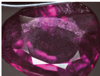
Figure 34: Reflective dendritic features are visible within the cement used to assemble the doublet. These features are responsible for the sheen-like reflections shown by this synthetic ruby doublet. Photomicrograph by Sandeep Vijay; magnified 32 \times .
