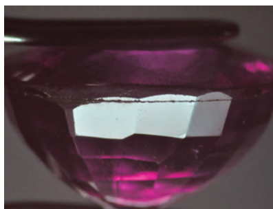
Figure 35: The junction plane of the synthetic ruby doublet is positioned just below the girdle. Photomicrograph by Sandeep Vijay; magnified 32 \times .
