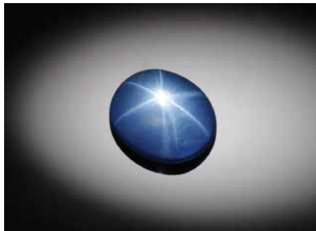
Figure 25: This 7.65 ct imitation resembles a star sapphire, but actually consists of colourless natural star quartz with an amorphous blue coating on the base of the cabochon. Photo by Bilal Mahmood.
