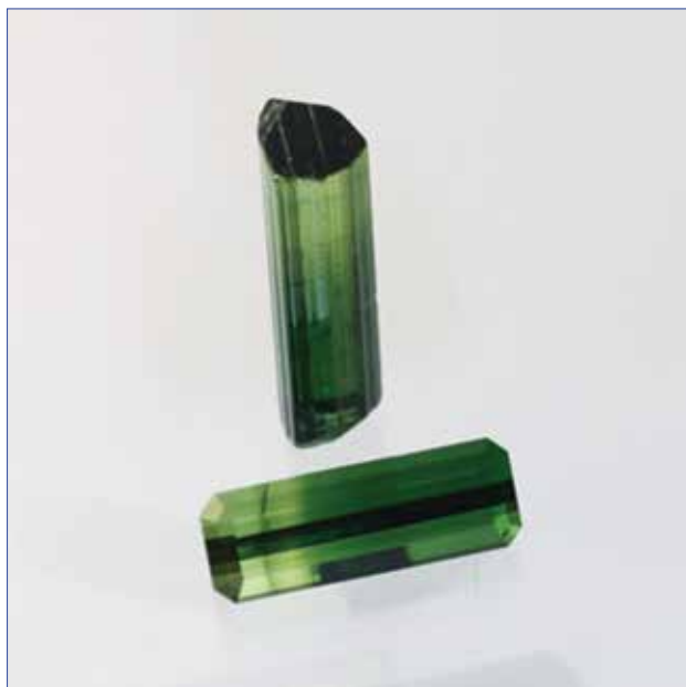
Figure 10: These rough and cut Cr- and V-bearing tourmalines show distinct colour zoning perpendicular to the c-axis. The crystal is ~21 mm long and the cut stone weighs 6.11 ct. Photo by B. Williams.
