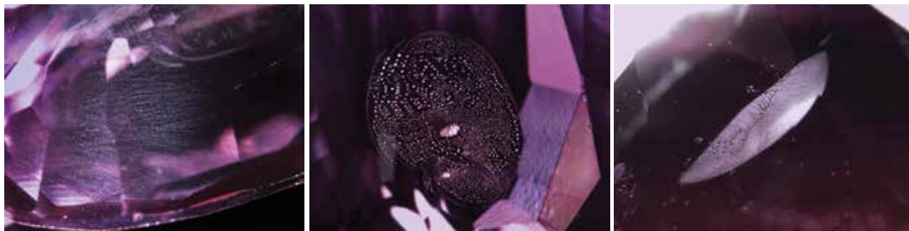
Figure 28: Various thermally altered internal features were present in the Cr-diffused sapphires, confirming their natural (not synthetic) origin. These include lines of stringers composed of fine rutile particles (left), negative crystals with associated partially healed stress fractures (centre) and partially healed fissures with a frosted appearance (right). Photomicrographs by C. P. Smith; magnified 40× (left and centre) and 62× (right).
