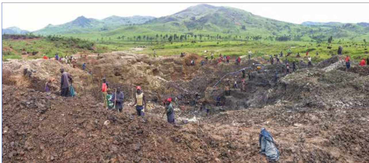
Figure 7: This open pit near Numbi, DRC, is being excavated with hand tools to reach an alluvial layer containing gem tourmaline and columbite-tantalite minerals. Photo by Farooq Hashmi.
