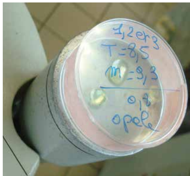
Figure 9: The measurement geometry used to assess the radioactivity of the hyalite is shown here. The three fashioned samples (0.83–1.81 ct) are positioned face-down on the detector. Photo by Michael Bailly.
