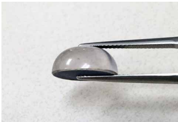
Figure 26: In profile view, it became apparent that the cabochon in Figure 25 is actually colourless. The blue colour viewed face-up is due to a coating on the bottom of the cabochon. Photo by Kelly Kramer.
