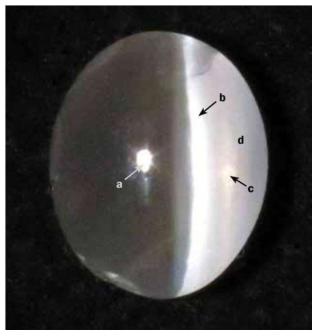
Figure 2: The 2.18 ct cat's-eye sillimanite is shown with fibre-optic illumination coming from 15^\circ to the left of vertical, and viewed from directly above. The chatoyancy-causing fibres are oriented parallel to the base and to the shorter axis of the cabochon. Photo by H. Killingback. The labels refer to the discussion in the text.
