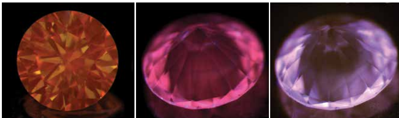
Figure 2: The luminescence exhibited by the 1.6-mm-diameter sample under three different broadband UV excitations is highly unusual for a colourless diamond. The ‘greenish’ orange (under 250–350 nm excitation), pink (355–375 nm excitation) and purple (300–410 nm excitation) luminescence with a slight streakiness are very good indicators of its CVD synthetic origin. Photos by F. Notari (left) and T. Hainschwang (centre and right).
