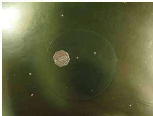
Figure 12: This example of the 'Heart of Pearls' marking technique shows an octagonal tag measuring 400 µm across that is glued to the surface of a Pinctada margaritifera cultured pearl. The tag is inscribed with 'A.BCD', which is clearly visible with a gemmological microscope. The tag is surrounded by a hardened layer of colourless transparent glue. Photomicrograph by O. Segura.
