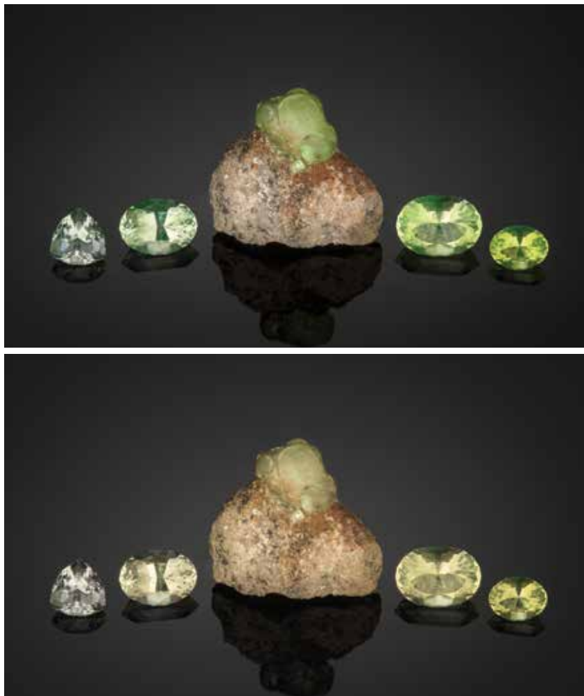
Figure 1: This matrix specimen (2.5 cm wide) and the cut gemstones (1.34–3.93 ct) show the range of colour appearance resulting from green daylight-induced fluorescence in hyalite from a relatively new deposit in Zacatecas, Mexico. They have been photographed using daylight-equivalent strobe lights (top) and using incandescent modelling lamps within the same strobe fixtures (bottom). The gems were faceted by author MG. Photos by Orasa Weldon.
