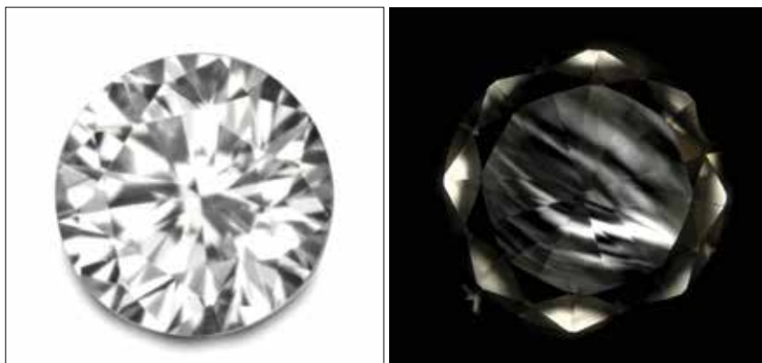
Figure 1: This 1.6-mm-diameter, F-colour, IF-clarity CVD synthetic diamond was found in a parcel of natural melee (left; photo by T. Hainschwang). Its lamellar appearance between crossed polarizing filters (here, shown immersed in methylene iodide) is typical of CVD synthetic diamond (right; photo by F. Notari).
