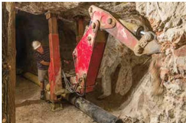
Figure 2: Deep underground at Lightning Ridge, Australia, miner Fred Mallouck operates a hydraulic excavator in search of black opal. Photo by Tino Hammid.
