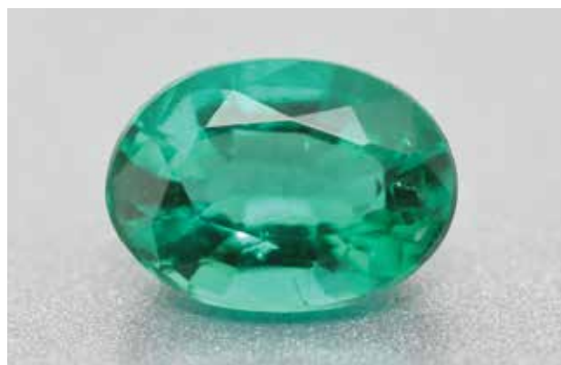
Figure 20: This 1.15 ct oval mixed cut proved to be a fracture-filled hydrothermal synthetic emerald. It was also unusual for its synthetic quartz inclusions. Photo by G. Choudhary.
