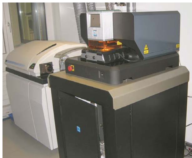
Figure 4: The instrumentation at the Gübelin Gem Lab used for this study consists of an ICP-MS (left side) and a laser ablation unit (right side). Photo by K. Link.
