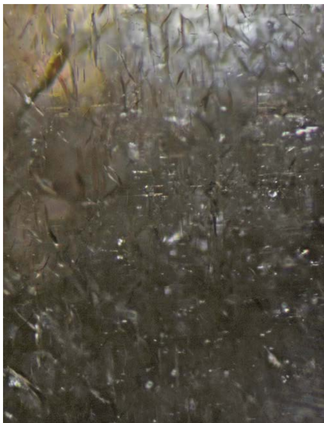
Figure 29: Microscopic observation showed that various micro-features are responsible for the star effect (left) and the central bright reflection (right) in the zircon. Photomicrographs © M. S. Krzemnicki, SSEF; magnified 75×.
