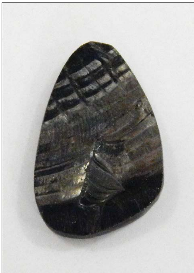
Figure 35: This 4.32 ct piece of shungite has been cut in a freeform shape, and the top surface has been left unpolished to show its conchoidal fracture patterns. Photo by Pangemtech staff.
