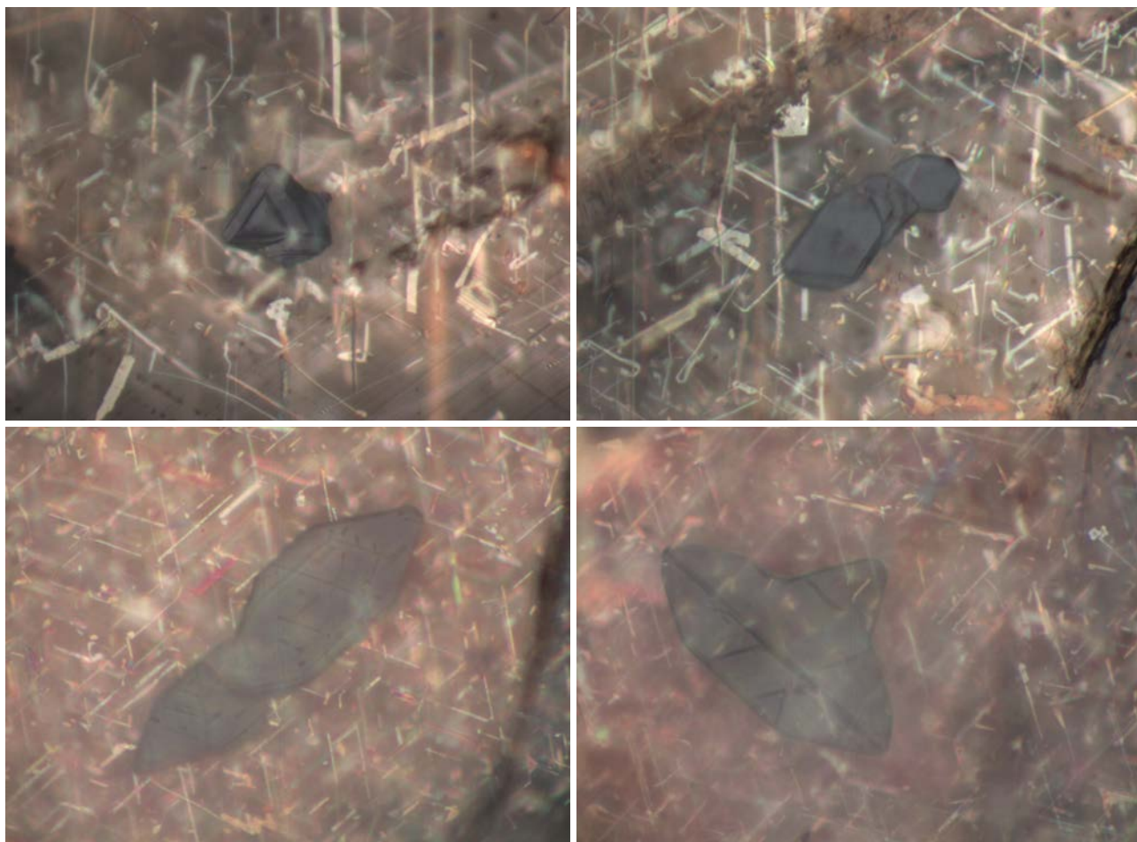
Figure 13: Black plates in the Gold Sheen sapphires were identified as magnetite. The edges of the inclusions are aligned along the first- and second-order hexagonal prisms. Photomicrographs by T. N. Bui using brightfield illumination; magnified 500× or field of view 175 × 130 μm (top left, top right and bottom left) and 1,000× or 80 × 60 μm (bottom right).
