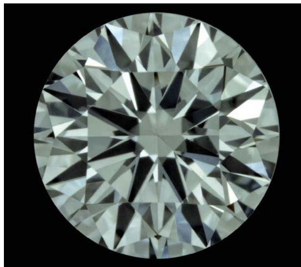
Figure 1: This 0.61 ct CVD synthetic diamond was submitted to NGTC without disclosure. Photo by Y. Lan.
