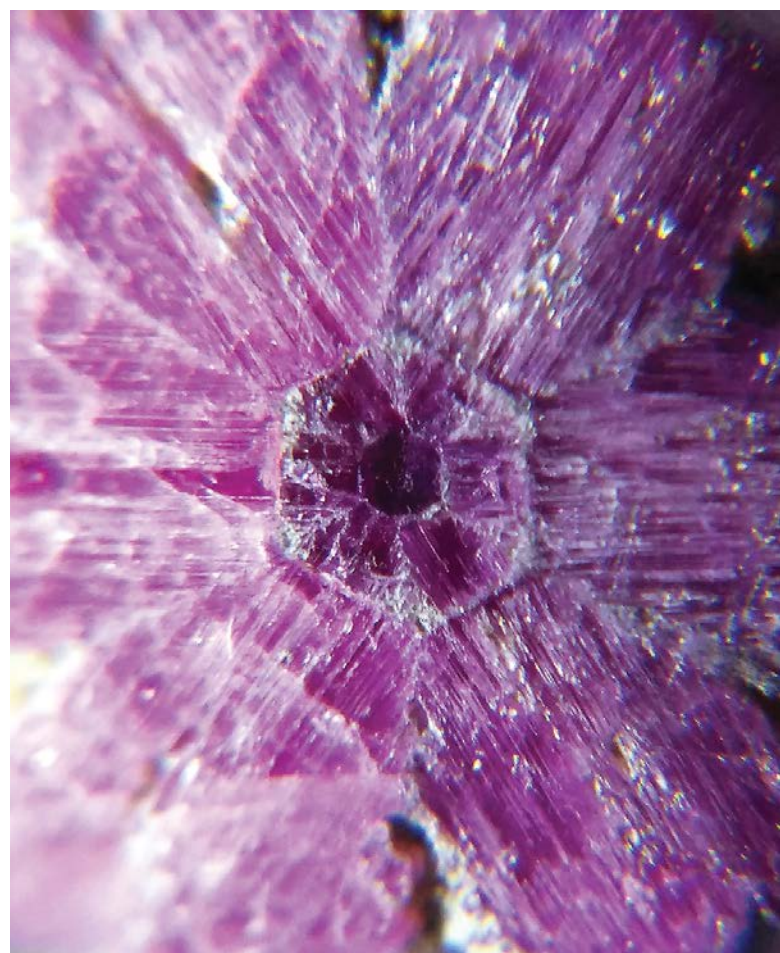
Figure 12: With magnification, this trapiche ruby displays a structure formed by three layers with different growth characteristics: a small deep red core, a middle layer with six arms/branches and an outer petal-shaped zone. Photomicrograph by E. Liu; magnified 15×.
