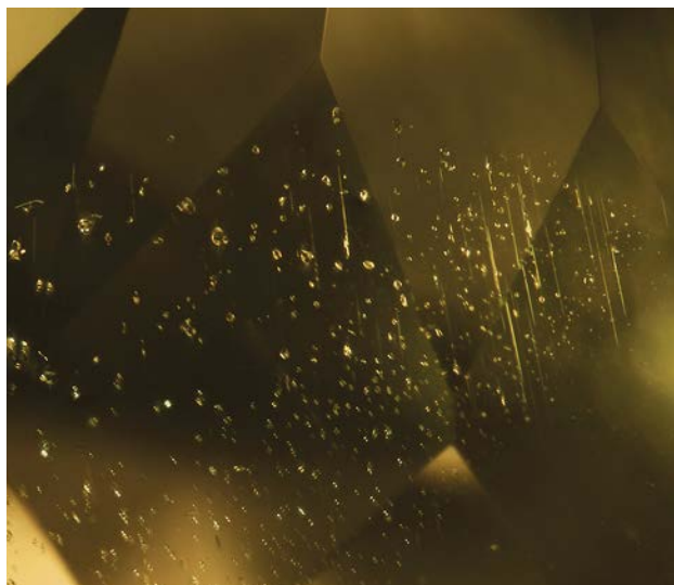
Figure 4: A parallel array of needle-like inclusions is present within a 'fingerprint' in a chondrodite reportedly from Tanga, Tanzania. Photomicrograph by Christopher P. Smith; magnified 68×.
