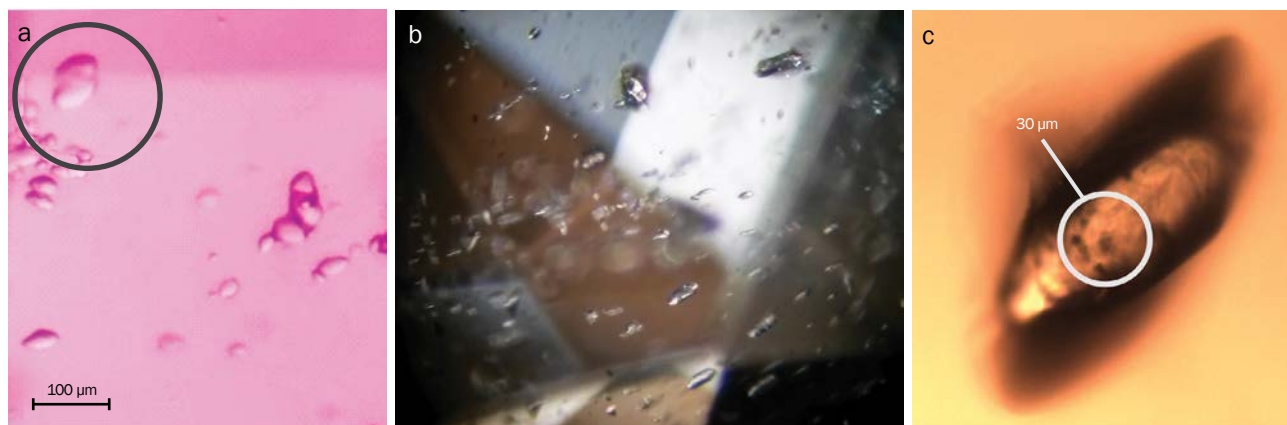
Figure 3: (a) In this cluster of zircon inclusions within the pink sapphire, the surface-reaching zircons that were analysed for age determination are circled. (b) Internal features in the greenish blue sapphire consist of isolated zircon crystals (top-centre and top-right), among other inclusions. (c) This zircon inclusion in the greenish blue sapphire was used for in situ age determination; the circle marks the position and size of the applied laser pit. Photomicrographs (a) and (c) by Klaus Schollenbruch, GGL; (b) is courtesy of Bulgari, image width ~2 mm.
