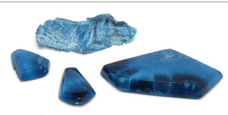
Figure 16: These samples from the DRC, consisting of a mixture of shattuckite and bisbeeite, were examined for this report. The slab weighs 19.91 ct, the flat cabochons are 3.14 and 3.61 ct, and the rough piece weighs 2.58 g. Gift of Kosnar Gem Co.; photo by Dirk van der Marel.
