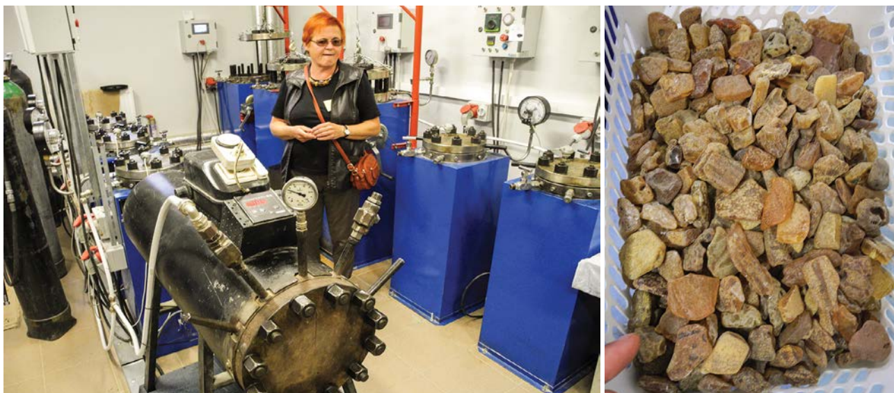
Figure 31: At the Amber Queen processing facility, autoclaves (left, with tour leader Sigita Pevceviute) are used to clarify the raw amber (right). Photos by B. M. Laurs.
