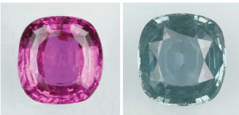
Figure 2: These pink and greenish blue sapphires (each ~12 ct) were submitted to the Gübelin Gem Lab in 2015. Both sapphires had surface-reaching zircon inclusions on their girdles, so age determination could be conducted. Photos by Janine Meyer, GGL.
