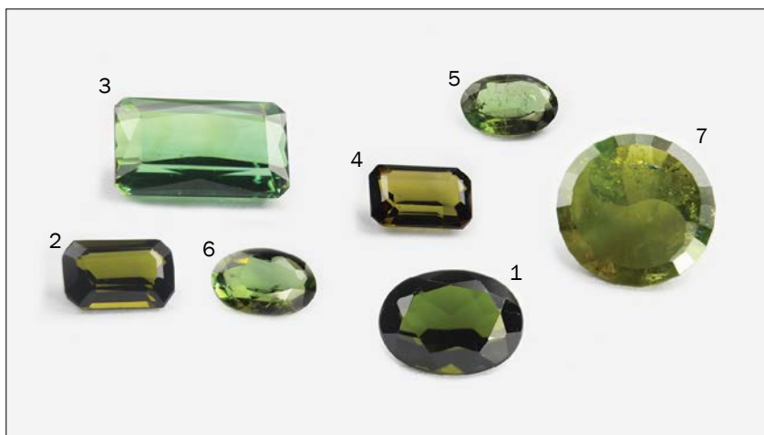
Figure 1: Of the green tourmalines shown here (0.53–2.74 ct), only one (no. 1) showed the Kerez effect in the refractometer. See Table I for RI data corresponding to each stone. Photo by Henry Mesa.
