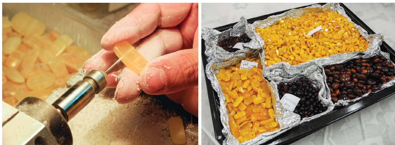
Figure 32: Hand drilling of amber pieces from both sides requires experience and concentration (left). Either before or after drilling, much of the amber undergoes heat treatment to darken its colour or create an ‘aged’ appearance (right). Photos by B. M. Laurs.
