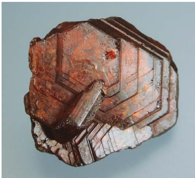
Figure 25: This wurtzite crystal (1.7 × 2.5 cm) from Merelani, Tanzania, shows a typical hexagonal habit. J. Hyršl collection and photo.
