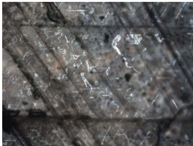
Figure 4: The surface of the basal pinacoid in this particular rough sapphire exhibits growth lines in three directions, parallel to \{10\bar{1}0\} . The needle inclusions below the surface are parallel to these growth lines. Photomicrograph by T. N. Bui using brightfield illumination; magnified 100 \times , field of view 860 \times 635 \mu\text{m} .
