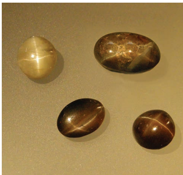
Figure 11: In these four-rayed star chrysoberyls, presumably from Sri Lanka, the b-axis of the crystals is almost perpendicular to the base of the cabochons. The weight of the samples ranges from 4.49 to 10.37 ct, and the cabochon at the lower right weighs 6.25 ct and measures 9.6 × 9.3 mm. A slice of the cabochon in the upper right was used for the preparation of two thin sections (sample D). Incandescent light, photo by K. Schmetzer.
