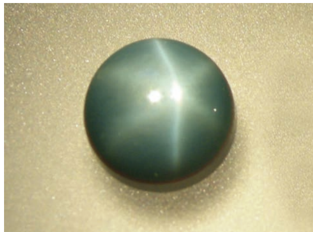
Figure 8: This six-rayed asteriated synthetic alexandrite produced by Kyocera weighs 1.63 ct and measures 8.3 mm in diameter. Daylight, photo by K. Schmetzer.
