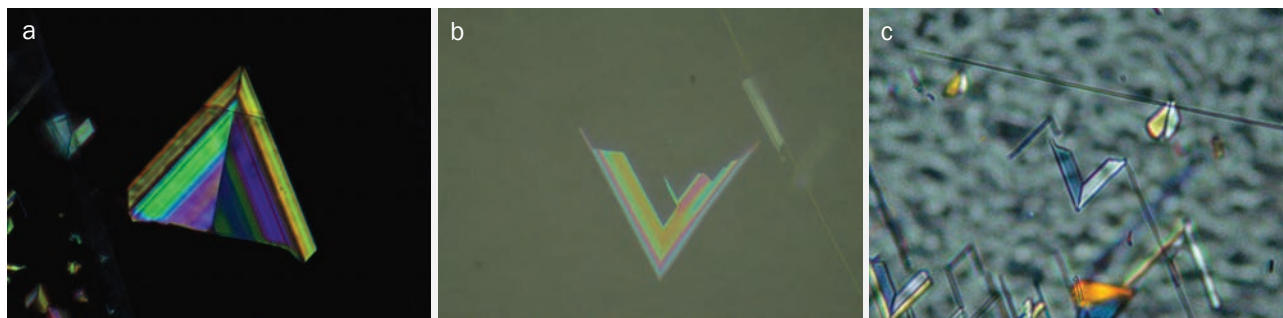
Figure 19: Somewhat larger V-shaped or triangular rutile platelets in the alexandrite from Kerala, cut perpendicular to the a-axis (sample C), are shown in these images (a, b and c). View parallel to the a-axis, reflected light, crossed polarizers, field of view 112 \times 84 \mu\text{m} ; photomicrographs by H.-J. Bernhardt.
