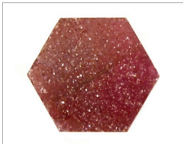
Figure 22: This polished hexagonal plate (3.32 ct) of ruby from Liberia displays abundant sparkles in reflected light that are due to reflections from rutile inclusions and polycrystalline grain boundaries. Photo by B. Williams.
