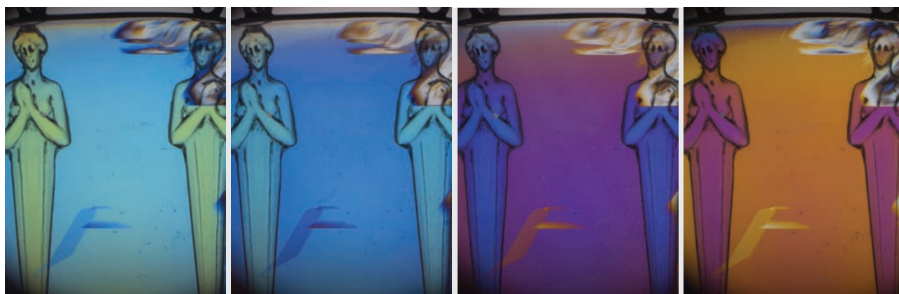
Figure 16: Different interference colours are also produced as the quartz pendant is rotated between crossed polarizers. Photos by C. Caplan; image width ~20 mm.
