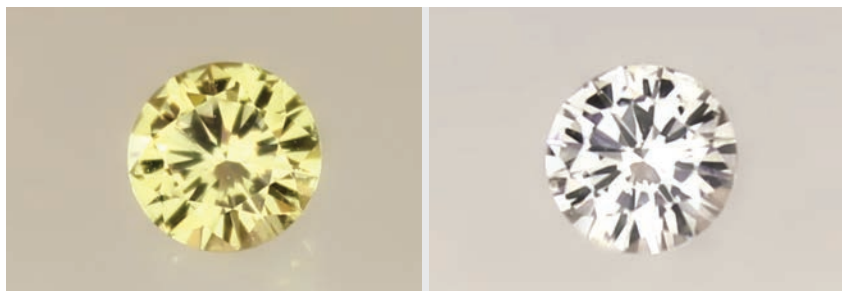
Figure 25: This 1.07 ct sapphire shows an unusual 'reverse' colour change. The more stable yellow state fades to colourless after low-temperature heating, and the yellow colour can be restored by exposure to long-wave UV radiation or daylight. Photos by B. Williams.
