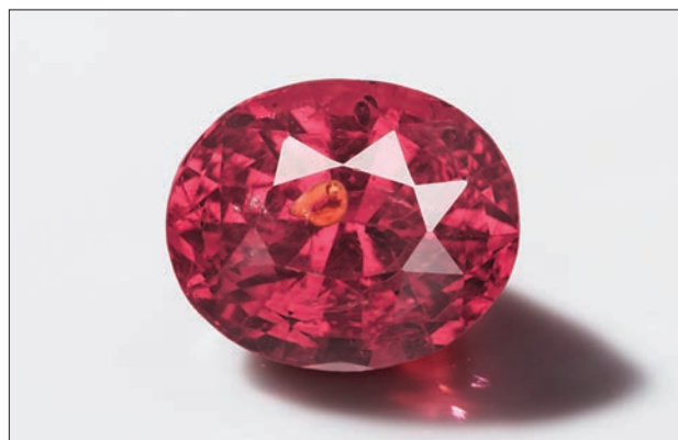
Figure 26: This 1.69 ct pink spinel, reportedly of Sri Lankan origin, contains a unique petroleum-bearing inclusion under the table facet. Photo by Bilal Mahmood.
