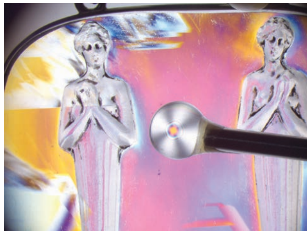
Figure 14: Viewed with crossed polarizers, the pendant shows a ‘bull’s-eye’ interference figure with the conoscope, as expected for quartz. Distorted Dauphiné twinning interference patterns are visible in the minor rhombohedron at top and left. Photo by C. Caplan; image width ~28 mm.
