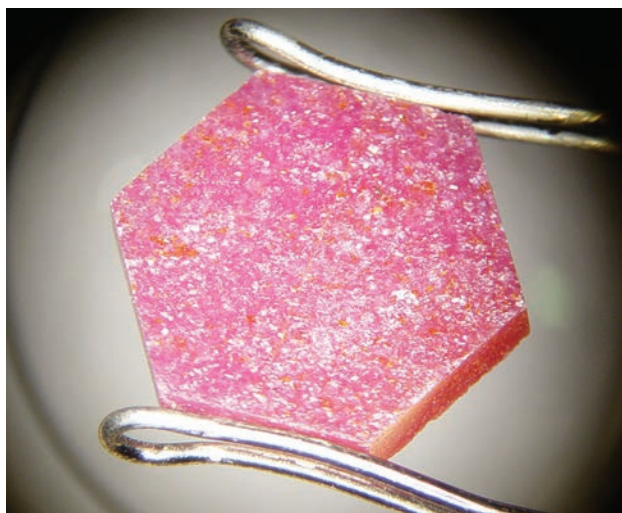
Figure 23: Seen here in oblique lighting, the 3.32 ct ruby shows a granular texture with orangey red domains corresponding to rutile inclusions. Photo by B. Williams.
