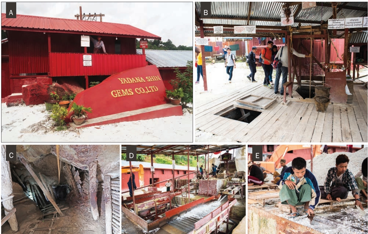
(A) Yadana Shin is one of the most well-known ruby mines in Mogok. (B) The mine workings are accessed by shafts, (C) which contain wooden ladders and timbering. (D) The mined material is passed through jaw crushers and then into jigs. (E) Workers sort the crushed rock by hand to recover the rubies. Photos by S. Saengbuangamlam (A, C) and T. Sripoonjan (B, D–E).
