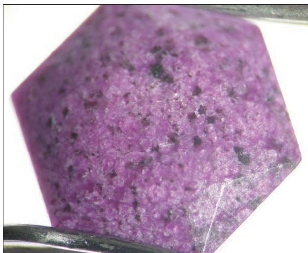
Figure 22: This stichtite (1.70 ct) was faceted from material that was mined in South Africa. The low lustre and rounded facet junctions visible at the lower right are consistent with the low hardness of stichtite. Gift of Mauro Pantò; photo by C. Williams.
