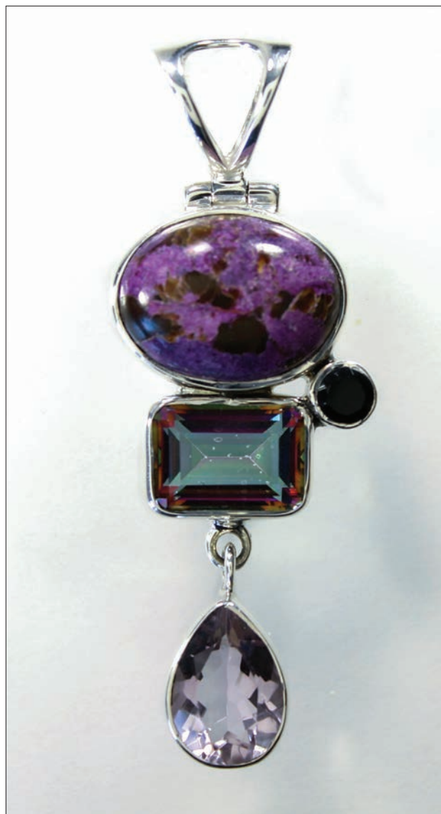
Figure 23: This pendant containing a 13 × 18 mm-wide cabochon of stichtite was submitted to Stone Group Laboratories in mid-2016. It also is set with pale amethyst, CVD-coated colourless quartz and black onyx, in sterling silver. Photo by B. Williams.
