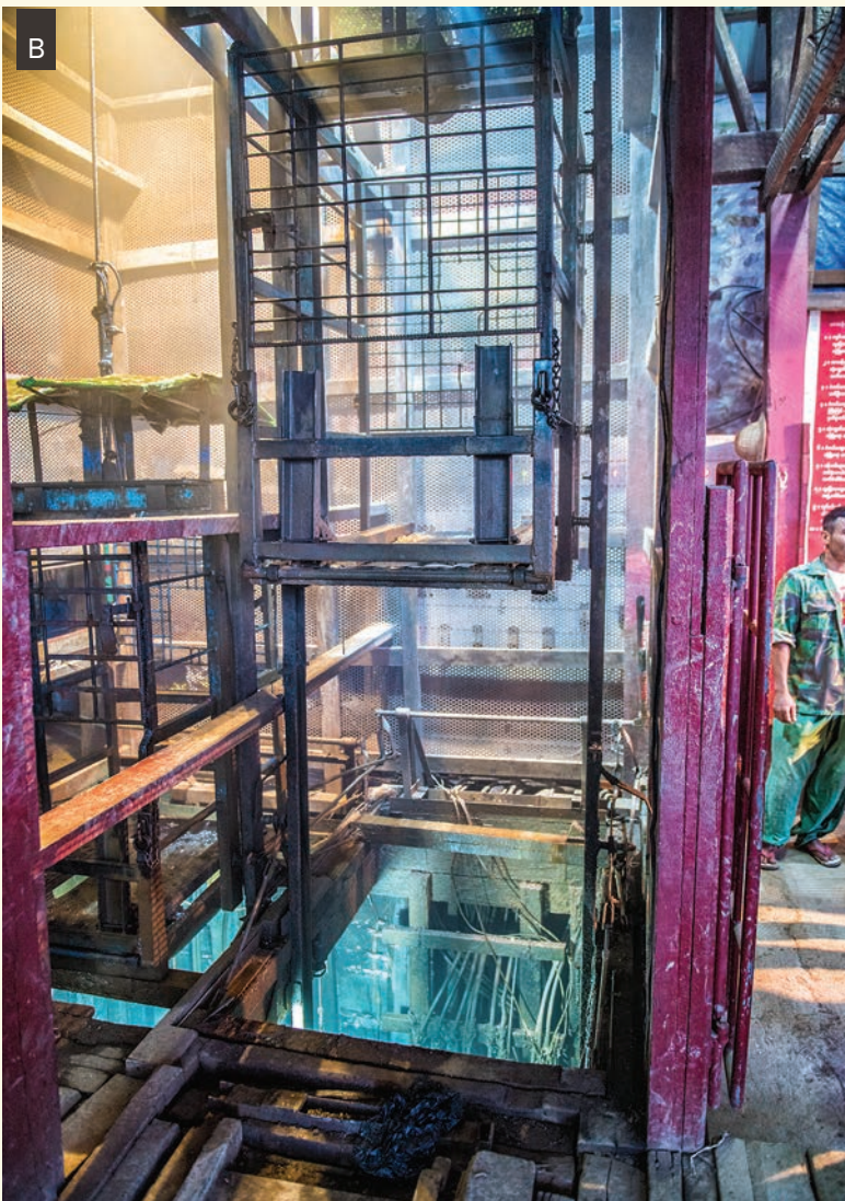
(A) The Ruby Dragon mine is surrounded by steep, forested slopes. (B) An elevator is used to access this Ruby Dragon shaft. (C) The mine manager shows a scale model of the underground workings. (D) The air in the shaft is hazy from the mining activities below. (E) Ore carts are used to bring the mined material to the surface. Photos by T. Sripoonjan (A–D) and S. Saengbuangamlam (E).
