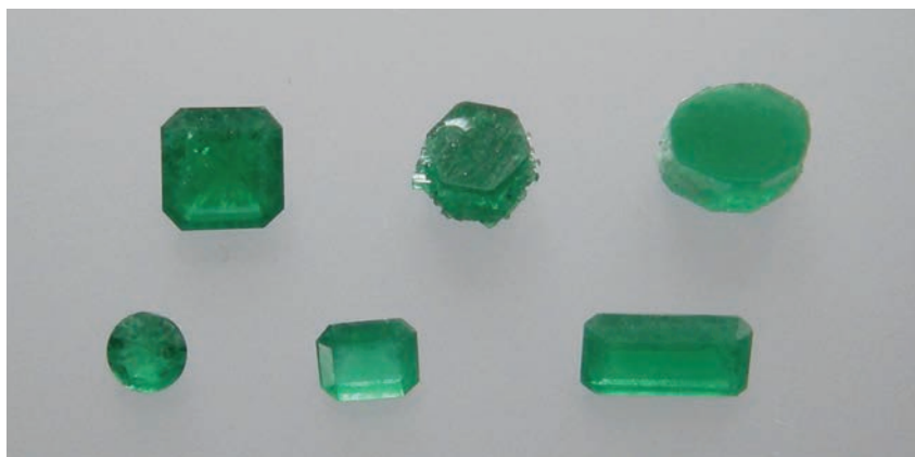
Figure 1: Shown here are faceted and rough synthetic emeralds grown by W. Zeffass in Idar-Oberstein, Germany, in the 1960s. The faceted samples weigh 0.24–1.02 ct, and the crystals are 0.23 and 0.40 g; the faceted sample on the upper left measures 6.4 × 6.4 mm and weighs 1.02 ct. Photo by K. Schmetzer.
