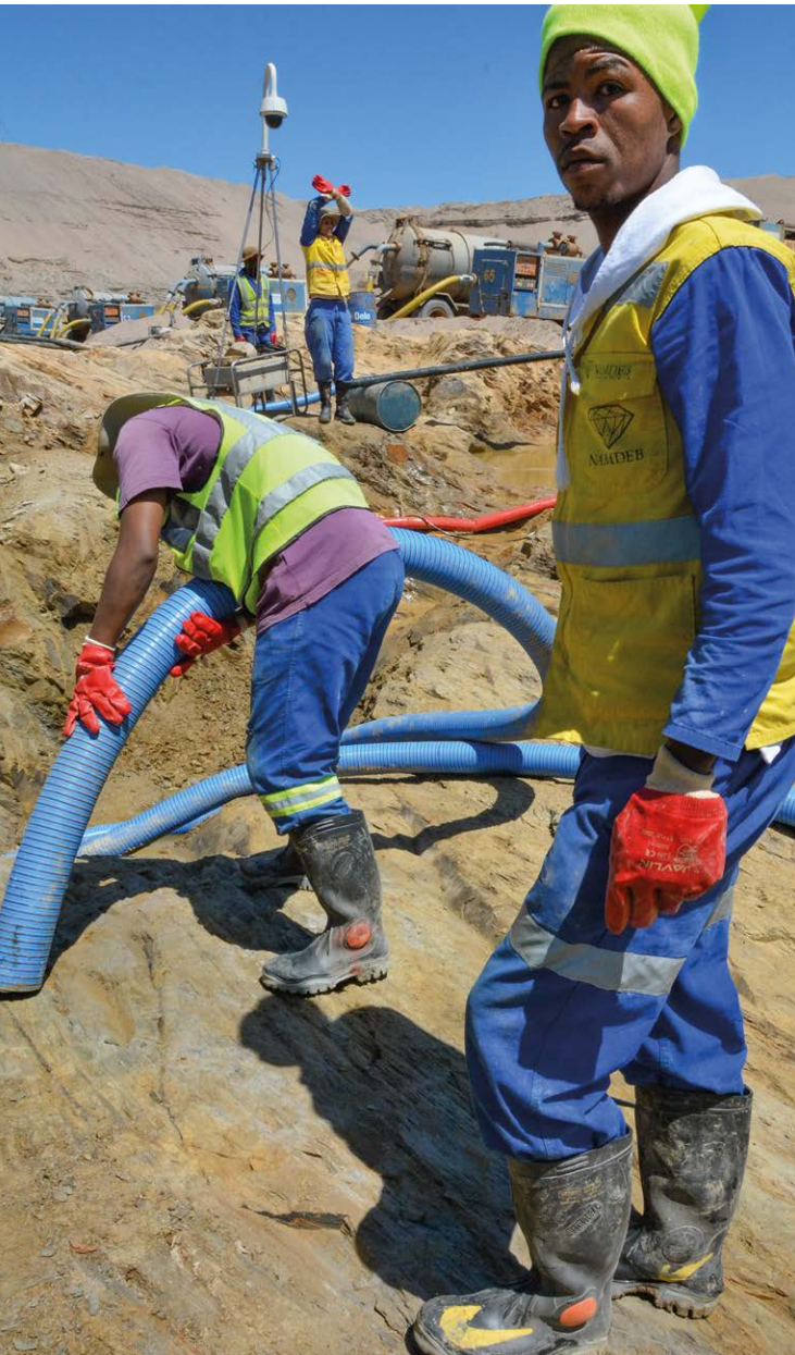
Figure 23: Members of the transvac crew work in pairs. They will stop vacuuming to pick up any diamonds that they see in the bedrock gullies, although such ‘pick ups’ typically occur only about twice per week. Photo courtesy of Namdeb.
