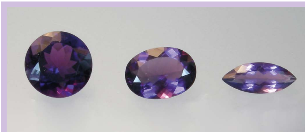
Figure 22: These amethysts, reportedly from ‘western Rwanda’, proved to contain intense violet growth zones twinned on the Brazil law. The samples weigh 19.72, 11.99 and 5.20 ct. Photo by K. Schmetzer.
