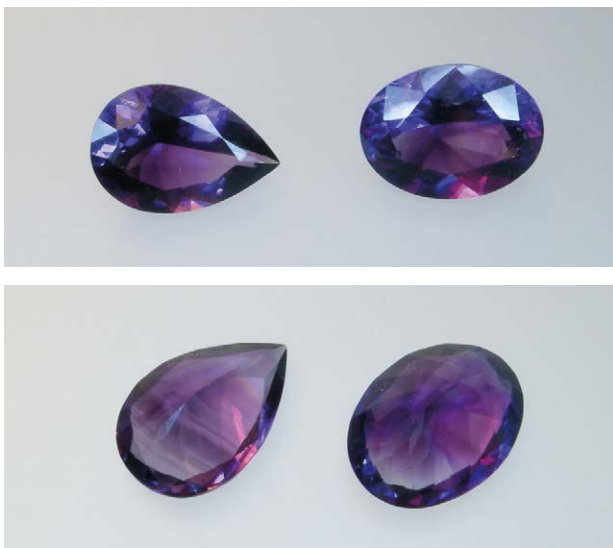
Figure 7: Faceted Rwandan amethyst commonly displays sectorial colour zoning, which typically consists of intense violet to purplish violet and lighter violet to almost colourless zones. The zoning may be visible in views toward the table facet (top), but it is more apparent in views toward the pavilion of the samples (bottom). The stones weigh 7.71 ct (left) and 10.03 ct (right). Photos by K. Schmetzer.
