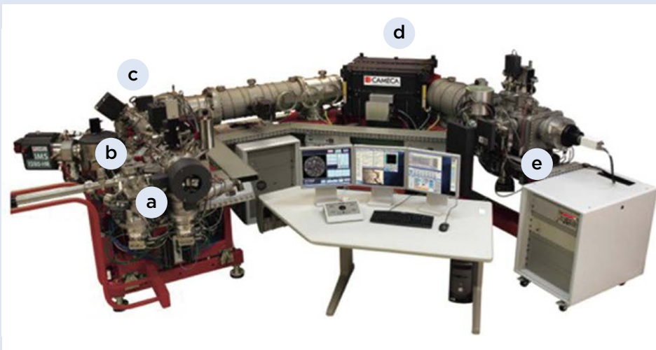
Figure 2: The SIMS instrument (Cameca IMS 1280-HR) at the SwissSIMS facility of the University of Lausanne consists of the following components: (a) sample chamber, (b) primary ion source, (c) electrostatic analyser, (d) magnet and (e) detection unit. Photo courtesy of SwissSIMS, University of Lausanne.
