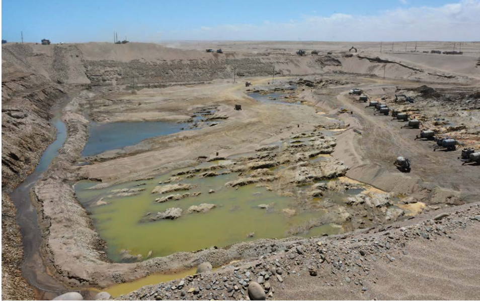
Figure 20: In October 2017, diamond mining was taking place at this pit in Namdeb's Southern Coastal Mines. The pit is flanked by sand walls, and ocean water is held back by the seawall to the far left. Previously mined bedrock gullies are visible in the centre of the photo, and on the right side is a series of transvac units and bins located adjacent to the current mining area. Photo courtesy of Namdeb.
