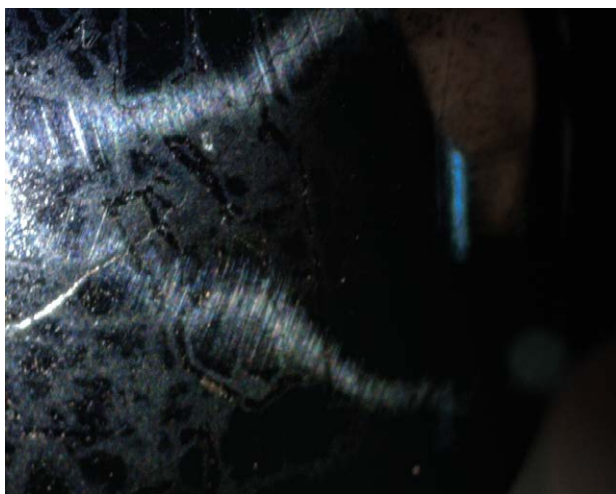
Figure 31: Parallel scratches on the surface of the 41.12 ct hematite-magnetite cabochon (shown here with two of the three orientations scratched on the sample) were responsible for its six-rayed star. Photo by B. Deljanin.
