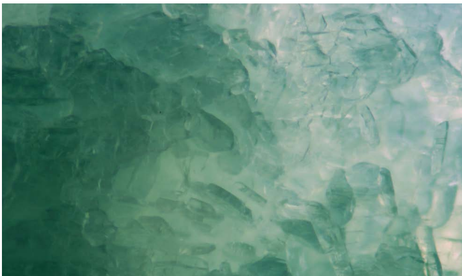
Figure 25: With magnification, tabular greenish blue sapphirine inclusions can be seen in the feldspar matrix of the grandidierite imitation. Photomicrograph by T. Stephan, transmitted light; field of view 2.8 mm.
