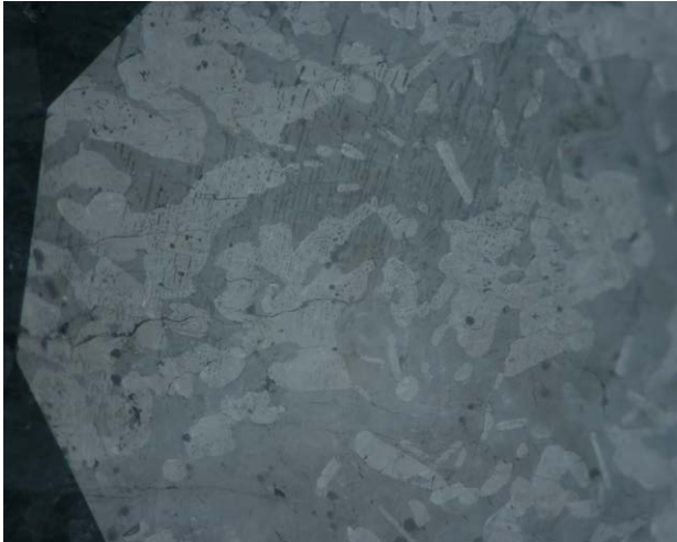
Figure 26: With reflected light on the table facet of the feldspar-sapphirine rock, the sapphirine inclusions show a brighter reflection than that of the plagioclase matrix. Photomicrograph by T. Stephan, reflected light; field of view 5.0 mm.
