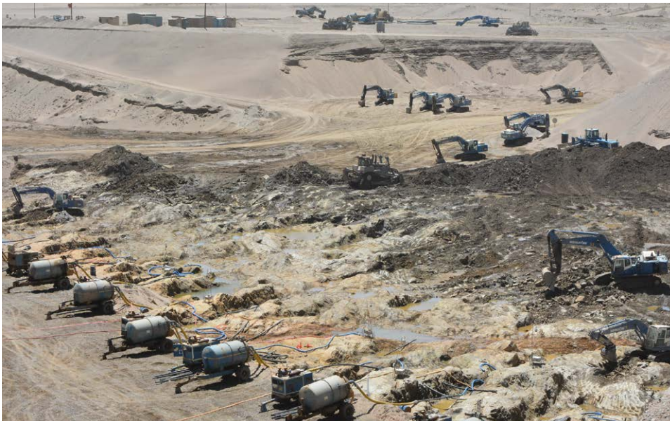
Figure 21: To recover diamond-bearing gravels from the bedrock trappsites, excavators and bulldozers first remove overlying sediments, as well as some areas of the bedrock itself, and then transvac machines (each with an accompanying bin) are used to vacuum any remaining sediments from the bedrock surface. Photo courtesy of Namdeb.
