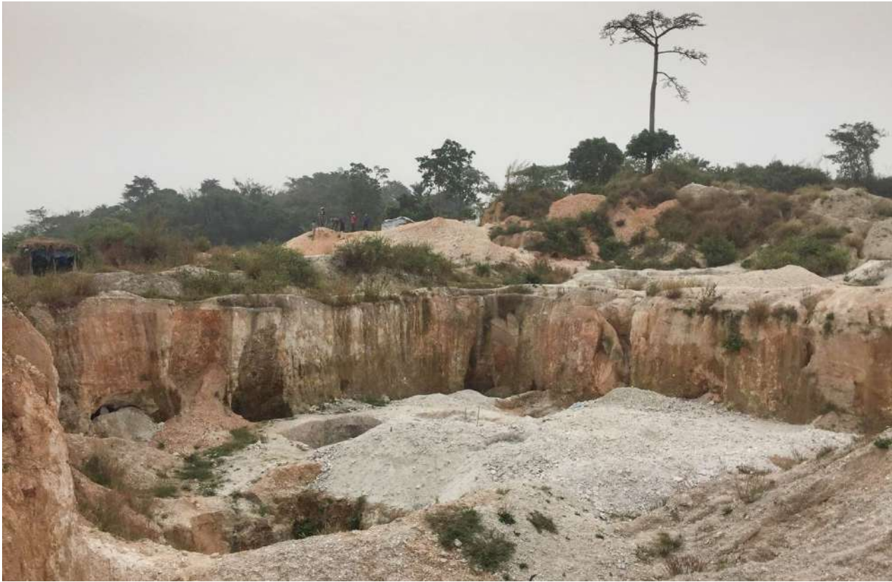
Figure 30: Miners have removed eluvial material from this pit in the Ijero area of south-western Nigeria in search of gem tourmaline. Photo by Farooq Hashmi.
