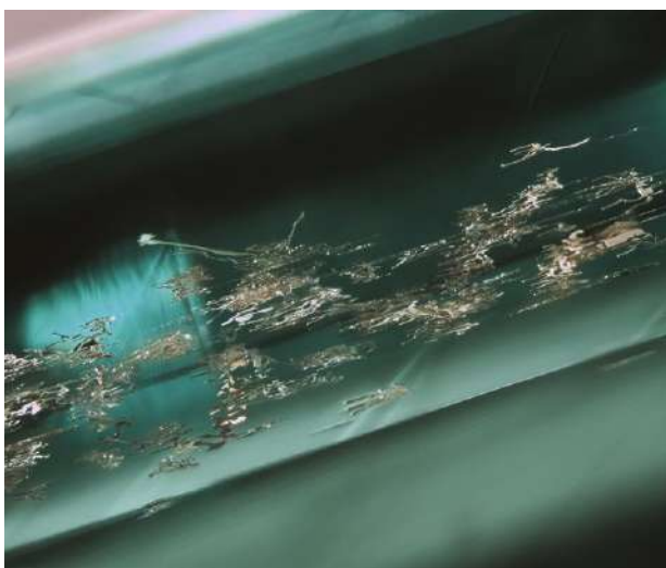
Figure 29: Dendritic platelets of native copper are oriented primarily along the c-axis of this Cu-bearing tourmaline. Photomicrograph by Bilal Mahmood; magnified 58x.
