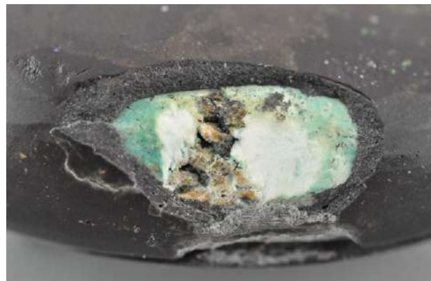
Figure 42: The chipped edge of one of the imitation matrix opals reveals the underlying magnesite used as the core, which was coated with a thick layer of granular grey cement. Also note the blue-green rim and white centre of the core, which suggests the local presence of dye in the magnesite. Photo by G. Choudhary.
