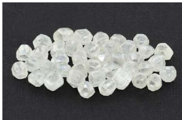
Figure 1: These near-colourless melee-sized rough synthetic diamonds (2–3 mm each) were grown in China. Photo by Jianxin (Jae) Liao, © GIA.
