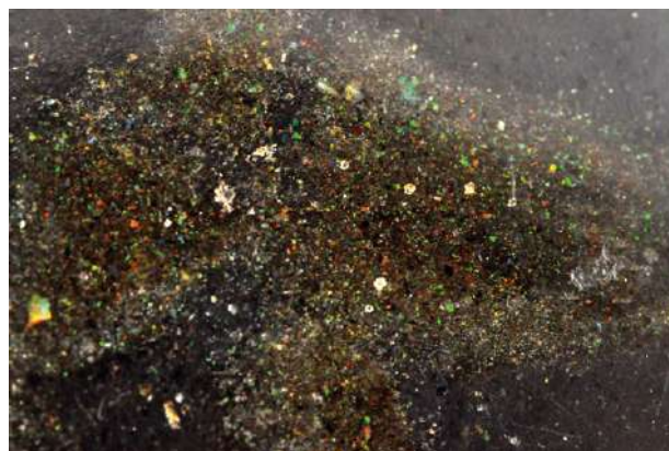
Figure 40: Grains showing play-of-colour are mainly restricted to the brown areas of this imitation matrix opal. They have been embedded into the top layer of grey cement. Photo by G. Choudhary.
