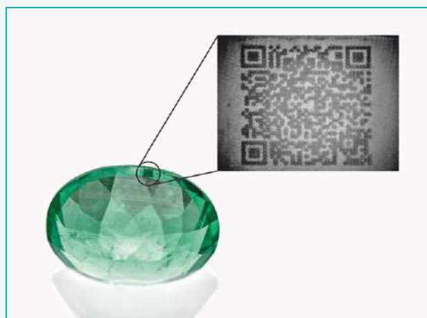
Figure 3: A tiny QR code can be inscribed on a gemstone during chemical analysis with GemTOF instrumentation (Wang and Krzemnicki, 2016). The QR code shown here measures 500 \times 500 \mu\text{m} and has been inscribed on the girdle of an emerald weighing 2.5 ct. The material ablated during the inscription of the code is used to measure trace-element concentrations that are evaluated for determining country of origin. The code can be read (after magnification) using a QR reader on a smartphone, and gives the user access to various types of information on the stone. Composite photo by H. A. O. Wang and V. Lanzafame, SSEF.
