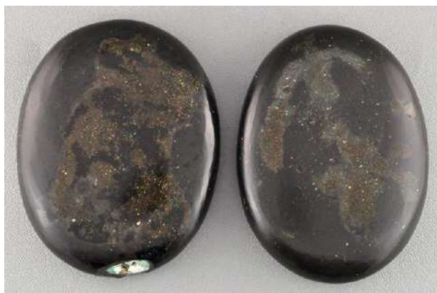
Figure 39: These two oval specimens, weighing approximately 750 ct each, were represented as black opal. They proved to be imitations made with a magnesite core coated with a layer of grey cement that locally contains tiny grains having the appearance of opal. The lower edge of the left specimen was chipped off for study. Also note the uneven colour patches, suggesting that different materials were used in their manufacture. Photo by G. Choudhary.
