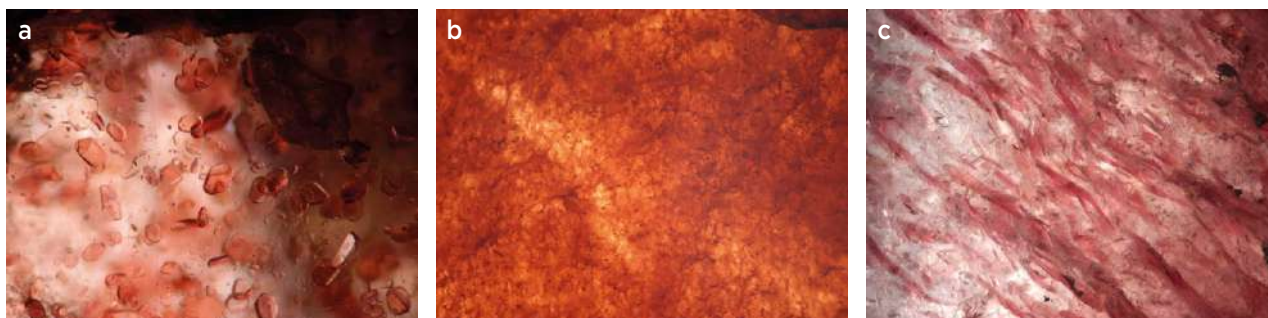
Figure 18: Polished slices of various types of red quartzite are viewed here in transmitted light. (a) The red aventurescent quartzite from Tanzania is coloured by muscovite inclusions. (b) In quartzite from India, the individual quartz grains are surrounded by thin films of hematite. (c) Quartzite from South Africa is also coloured by hematite, which forms platy, pink-to-red flecks oriented in one direction. Photomicrographs by T. Stephan; image widths 3.15, 7.14 and 3.32 mm, respectively.
