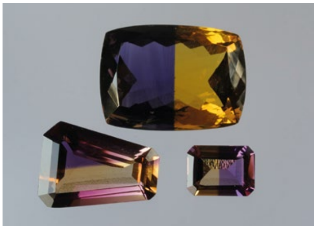
Figure 23: The glass imitation of ametrine (top, 28.98 ct) studied here displays darker colour and a sharper colour transition than two typical synthetic ametrines (9.62 and 2.62 ct). Photo by J. Hyršl.
