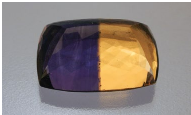
Figure 24: Viewed table-down, the 28.98 ct glass imitation of ametrine in Figure 23 shows colour zoning in the dark violet half and gas bubbles along the colour boundary. Photo by J. Hyršl.
