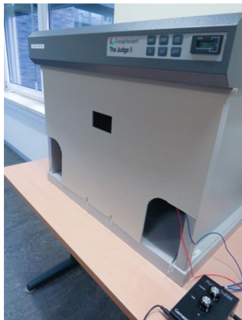
Figure 4: Left: A Gretag Macbeth Judge II cabinet is fitted with a UV LED array covered with a Wood's filter (black area next to the fluorescent tubes), and the diamonds are viewed in the tray that is raised above the base of the cabinet. A polycarbonate filter for the fluorescent tubes is not shown in this image. Right: The cabinet was modified for the observation experiments by fitting it with a front cover to exclude ambient light. Photos courtesy of HRD Antwerp.
