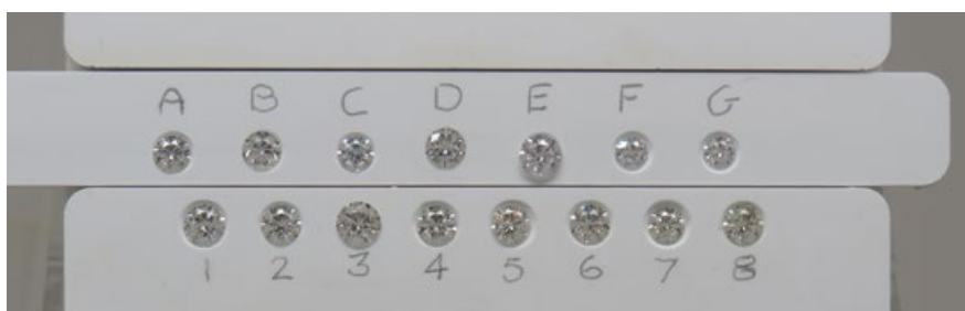
Figure 11: In Experiment 4, diamonds were observed table-up in order to evaluate the magnitude of any perceived colour difference in different lighting environments. The master set is numbered from 1 to 8, where 1 represents D colour and 8 is K colour. The series to grade is labelled A to G on a sliding strip. Photo courtesy of HRD Antwerp.
