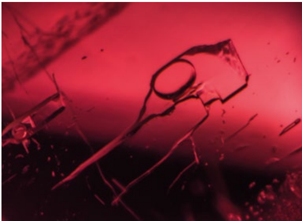
Figure 9: This two-phase (liquid and gas) fluid inclusion is present in a rhodochrosite from China (no. 4 in Figure 1). Photomicrograph by N. D. Renfro, image width 1.2 mm.
