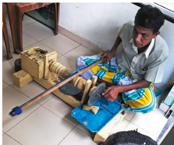
Figure 2: A Sri Lankan lapidary operates a traditional hanaporuwa in Ratnapura. The stone is held against a vertical lap, which is spun by drawing the bow back and forth. Photo by J. Prim.
