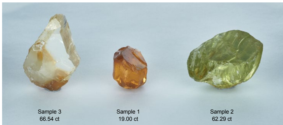
Figure 21: Although represented as being natural stones from a new discovery in Turkey, these samples were identified as synthetic periclase. Photo by Alex Mercado, AGL.
