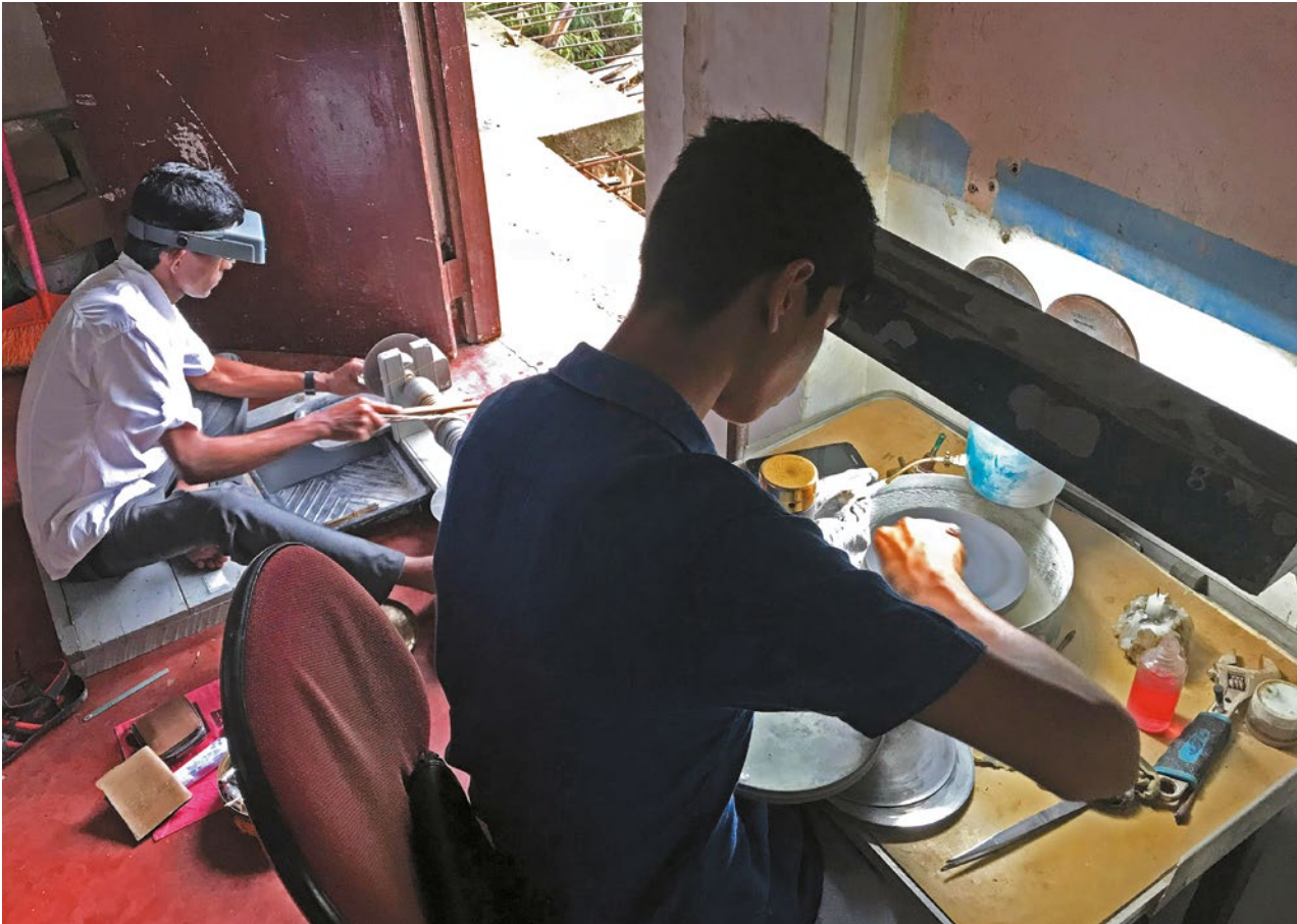
Figure 9: In this Ratnapura cutting shop, a traditional lapidary using a hanaporuwa works side-by-side with a modern cutter using a handpiece machine. Photo by J. Prim.
