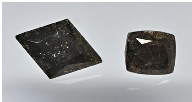
Figure 1: Anorthoclase from Antarctica (here, 2.29 and 1.61 ct) has a dark appearance due to the presence of abundant melt inclusions. Photo by Mauro Pantò.
