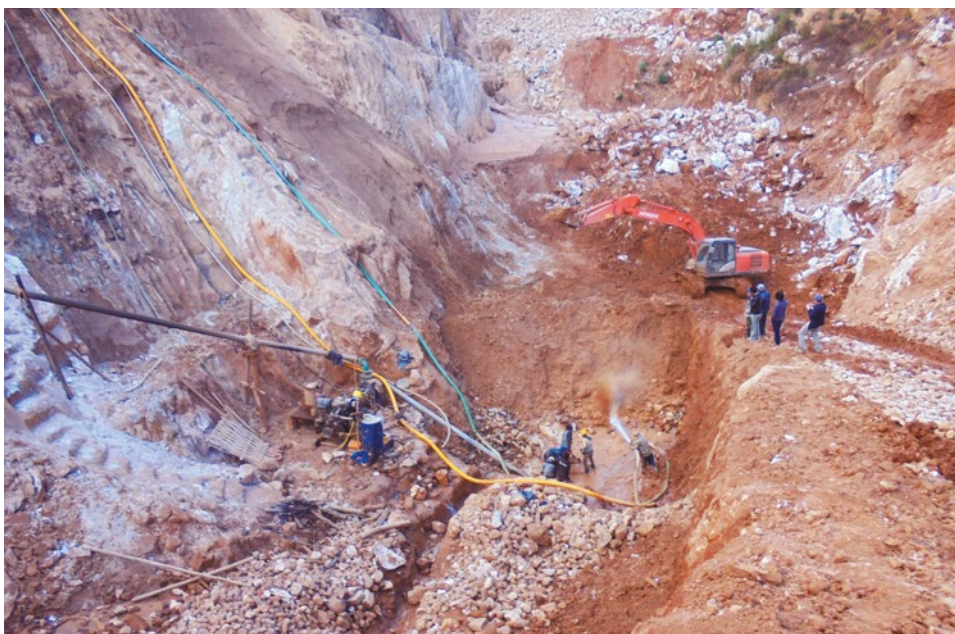
Figure 4: Hydraulic mining of gem-bearing gravels at Mansin in north-eastern Mogok demonstrates how spinels are obtained from secondary deposits. Photo © M. M. Phyo, 2016.
