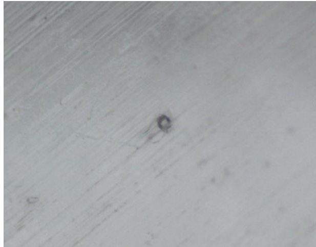
Figure 5: Examination with a gemmological microscope revealed this two-phase inclusion in the faceted blödite in Figure 4, which is seen here among prominent polishing lines. Because of the low hardness and the solubility of blödite, it is difficult to achieve a good polish. Photomicrograph by T. Stephan in transmitted light; image width 1.5 mm.
