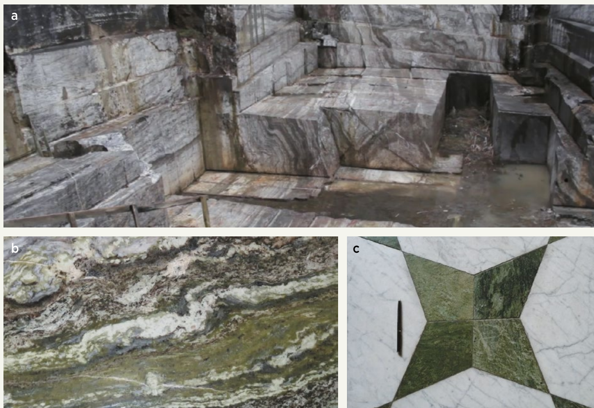
Figure 4: (a) In this photo of the Streamstown quarry, near Clifden, the folded and banded Connemara marble is clearly visible. This image is a frame taken from a LiDAR (light detection and ranging) survey of the quarry by McCaffrey et al. (2008). (b) A polished slab of Connemara marble (image width 30 cm) from the Streamstown quarry displays typical centimetre-scale banding and colour variations. (c) Streamstown Connemara marble inlays decorate the Carnegie Museum in Pittsburgh, Pennsylvania, USA (see pen for scale). Photos by M. Feely.
