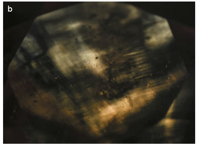
Figure 13: Microscopic examination of the 0.85 ct garnet reveals (a) angular graining patterns in shadowed transmitted light and (b) anomalous double refraction in cross-polarised light. Photomicrographs by N. D. Renfro, © GIA; image widths 3.57 mm.
