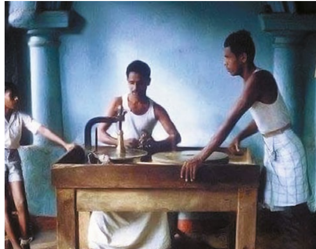
Figure 4: A lapidary polishes a stone with a bannku opa pattalaya machine, while an assistant turns the large wooden crank wheel. Photo courtesy of Ika Dayananda.
