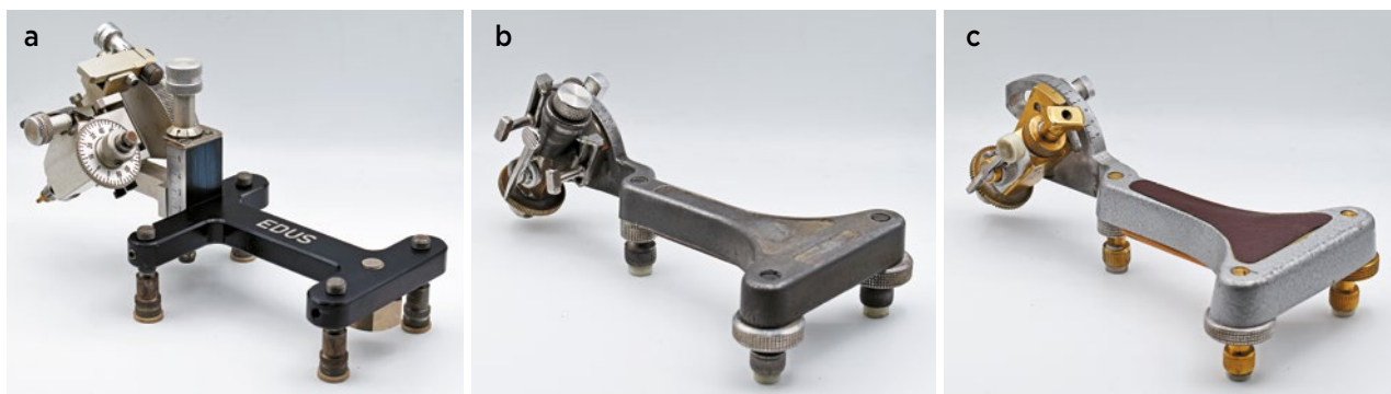
Figure 5: Shown here are faceting handpieces from EDUS (a), Imahashi (b) and Sterling Gems & Lapidary (c). Photos by J. Prim.
