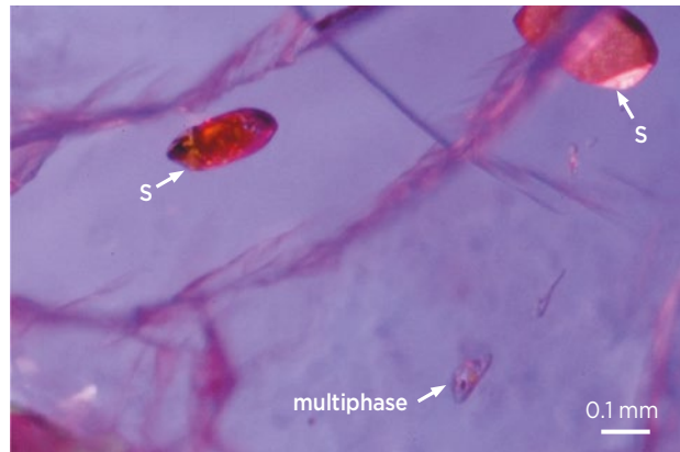
Figure 11: Solid inclusions of elemental sulphur (S) are seen here with multiphase fluid inclusions (probably containing liquid and sulphur) in a spinel from Mansin. Photomicrograph by M. M. Phyo.
