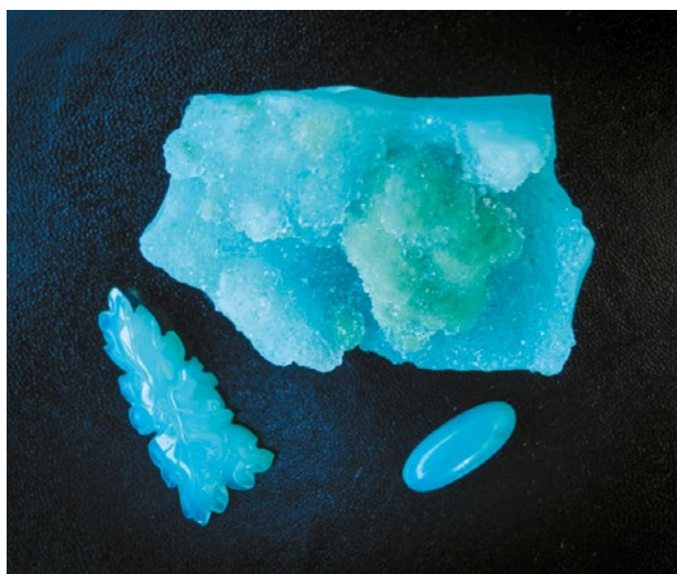
Figure 6: This rough specimen (68.0 mm long) and cabochon of chrysocolla were recently produced from the Ray mine in Arizona. Shown for comparison is a carving (27.4 mm long) made from high-quality chrysocolla that is from elsewhere in Arizona. The rough specimen is covered by drusy quartz, and the greener portion may correspond to the presence of malachite. Photo by B. M. Laurs.
