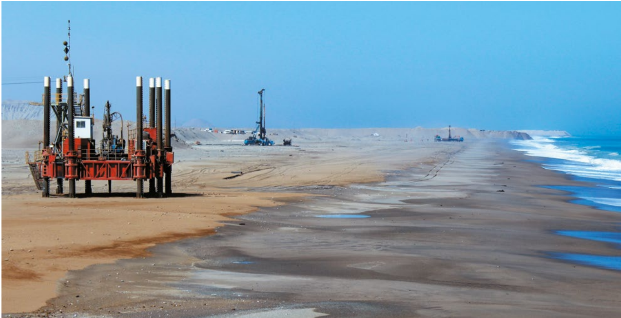
Figure 5: Three exploration tools currently being employed at the Southern Coastal Mines are visible here (left to right): a probe drill platform, a large-diameter sampling tool known as BG36 and a small-diameter sonic drilling tool. Photo by Edmund Nel.
