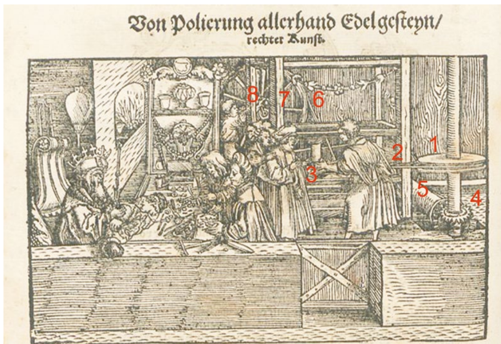
Figure 7: An apparatus for polishing gems was depicted in a book about plants, animals, gemstones and minerals written by Eucharis Röβlin in 1550. The large wheel used as the power source (7) is seen in the background, and the horizontal driving wheel (1) for the smaller polishing wheel is at the right. See text for an explanation of the numbers and parts. After Röβlin (1550).
