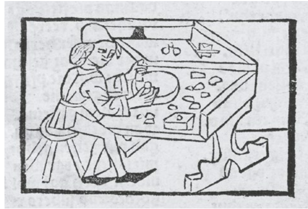
Figure 6: A disc for shaping and polishing gemstones was depicted in Volmar's Steinbuch (1498).
