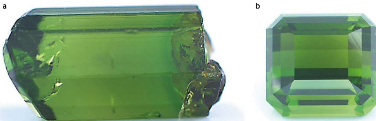
Figure 1: (a) The Commander mine in Tanzania is the source of this 14-mm-long tourmaline of pure green colour. (b) Faceting of this crystal by author CS yielded a 2.13 ct gemstone with the table oriented parallel to the c-axis. Photos by C. Schwarzingler.
