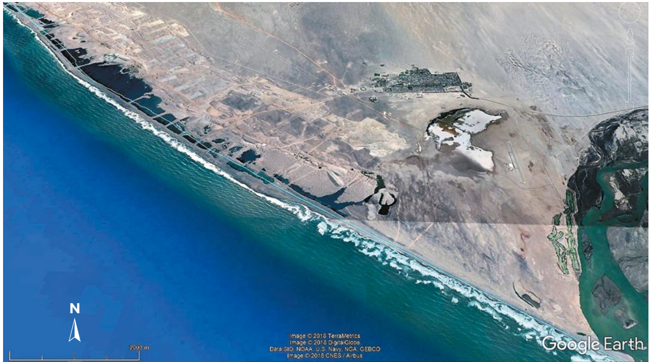
Figure 4: In this satellite image from Google Earth (imagery date 18 October 2017, viewed from approximately 7,660 m elevation), the high-water line for the year 2000 is shown in blue, illustrating areas where the land has been extended up to 500 m seaward since that time. A series of flooded mining pits are present along the coastline. The Orange River is visible on the far right, and the town of Oranjemund is seen as the dark area in the upper part of the image.
