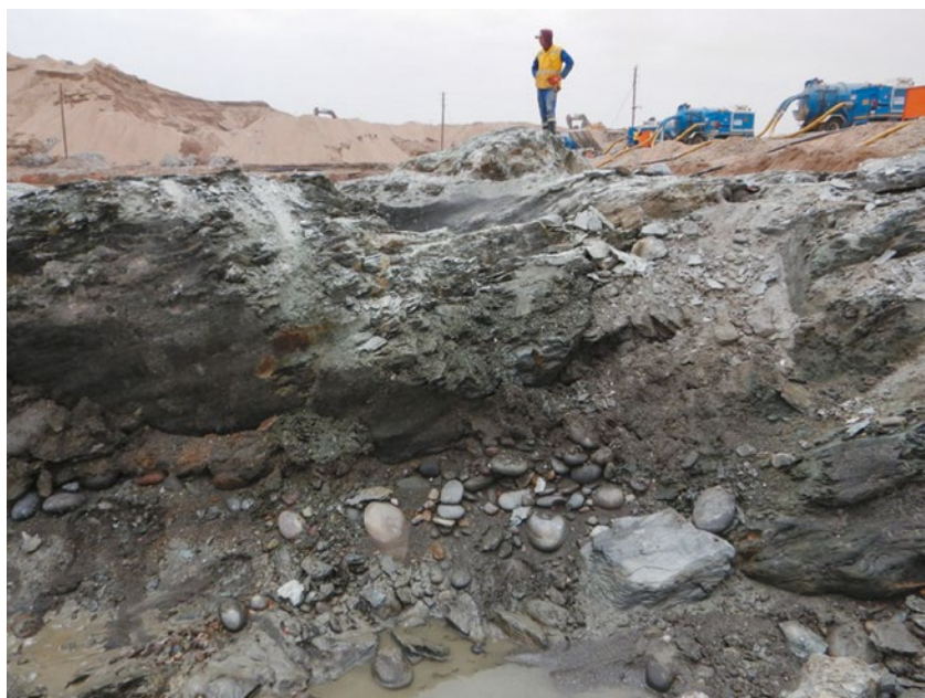
Figure 6: Diamondiferous marine gravel trapped in bedrock gullies has been exposed by the mining process. The rounded cobbles show where the gravel is located within a gully in the schist bedrock. The blue machines seen at the upper right are transvac units. Photo by Jennifer Nehoya.
