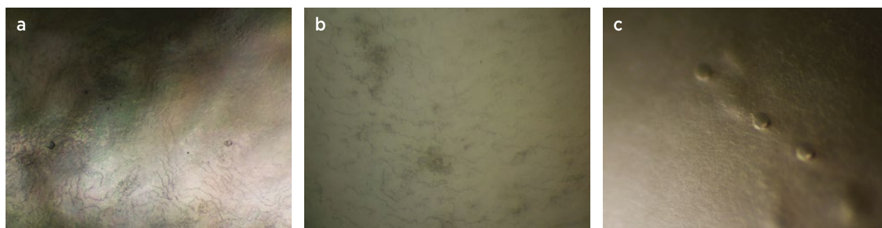
Figure 6: The typical appearance of overlapping layers of nacre is shown on the surface of (a) bead-cultured and (b) non-bead-cultured pearls. (c) Small bumps form blemishes on a bead-cultured pearl. Photomicrographs by Z. Ali; image widths 2.1 mm.
