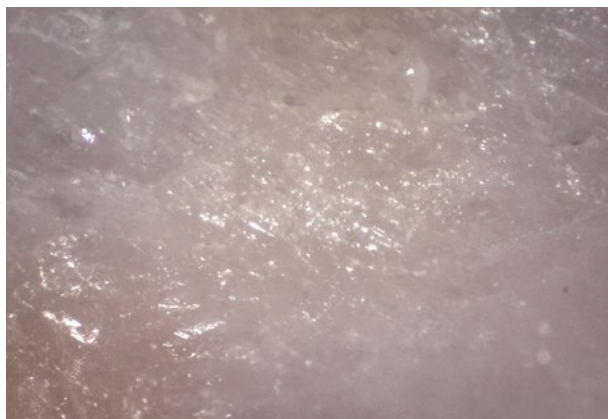
Figure 5: The cabochon in Figure 4 contains numerous tiny reflective fractures in a fairly consistent orientation that are responsible for its weak chatoyancy. Photomicrograph by Brendan M. Laurs; image width 1.0 mm.
