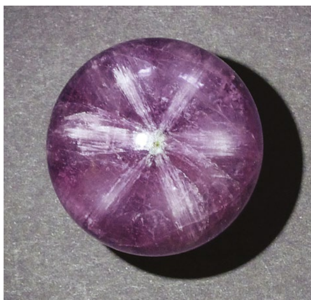
Figure 1: The 420.50 ct amethyst sphere described here displays a conspicuous whitish trapiche-like pattern. Photo by J.-P. Gauthier.
