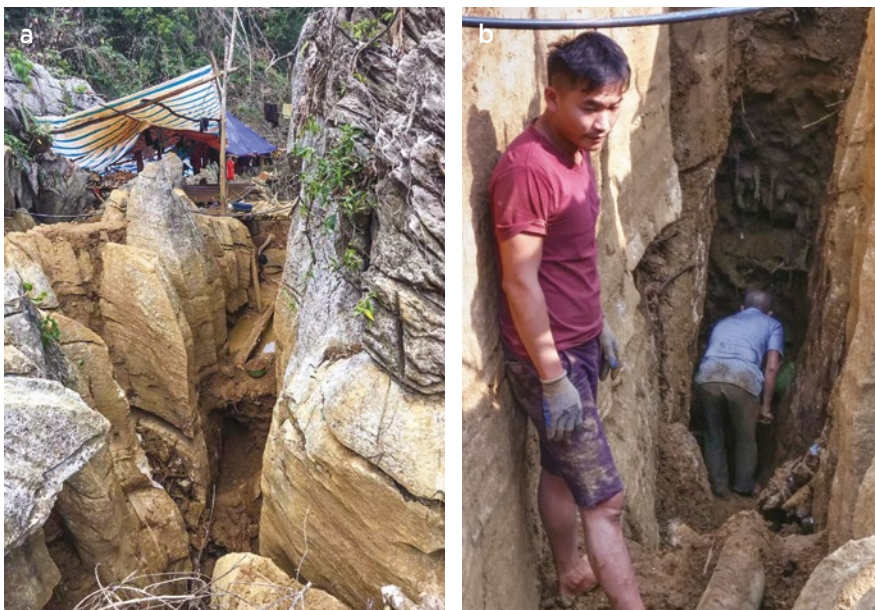
Figure 33: (a) The Bai Boui spinel mining area is situated in karst terrain. (b) Gravels containing blue spinel are mined from narrow ravines in the weathered marble. Photos by (a) D. Pisutadamongkol and (b) D. Blauwet.
