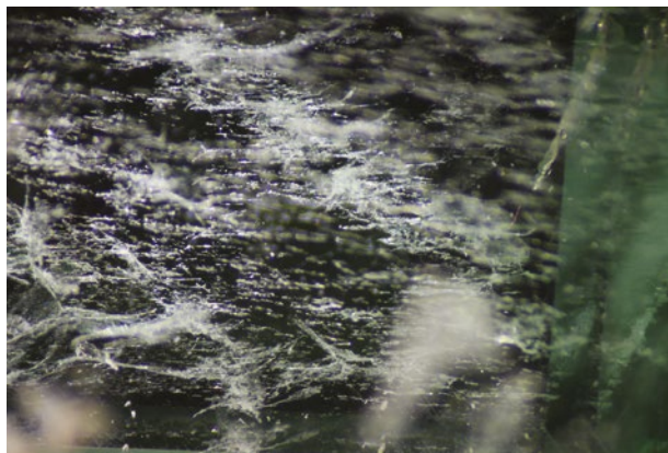
Figure 30: The cat's-eye effect in the Vietnamese orthoclase is caused by linear arrays of voids and channels. Photomicrograph by R. Hanus; image width 2.8 mm.
