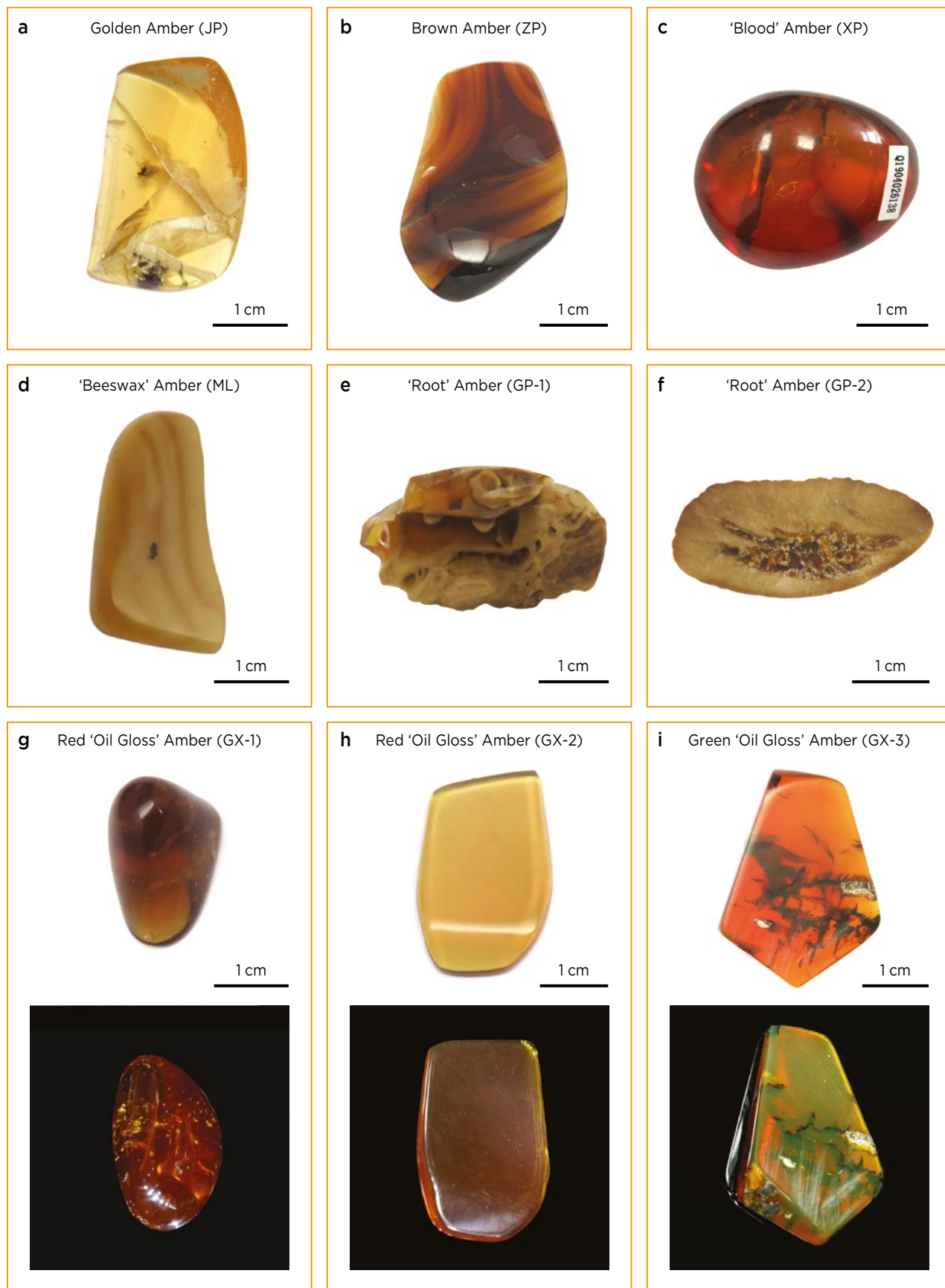
Figure 6: Burmese amber samples studied for this report include (a) golden, (b) brown, (c) 'blood', (d) 'beeswax', (e and f) 'root', (g and h) red 'oil gloss' and (i) green 'oil gloss' varieties. The colour appearance of the 'oil gloss' varieties is shown against both white and black backgrounds. Photos by X. Jiang.
