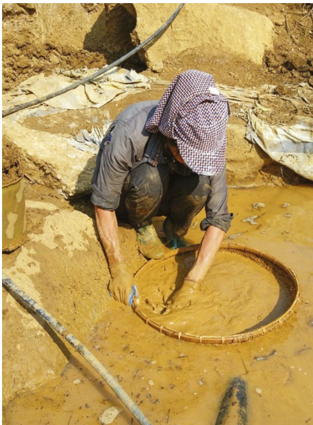
Figure 34: The spinel-bearing gravels are hand washed in a small pond using shallow baskets. Photo by D. Blauwet.
