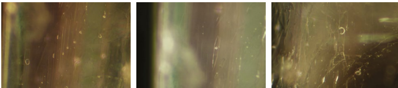
Figure 14: Two-phase (liquid-gas) inclusions displaying various shapes occur in the Diana Maria fluorites. Photomicrographs by J. Štubňa; magnified 40 \times .
