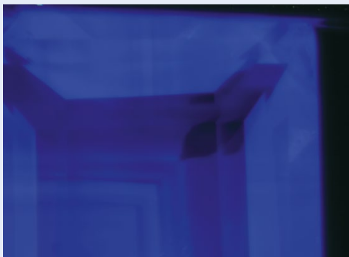
Figure 15: Intense violetish blue fluorescence is seen with long-wave UV radiation in this Diana Maria fluorite. Note also the subtle zones displaying magenta fluorescence. Photomicrograph by J. Štubňa; magnified 7.5 \times .
