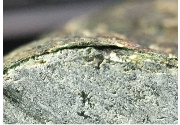
Figure 44: Slicing the sample reveals that the artificial crust consists of a waxy-looking exterior and an underlying green layer. Photomicrograph by W. Lu; magnified 15 \times .
