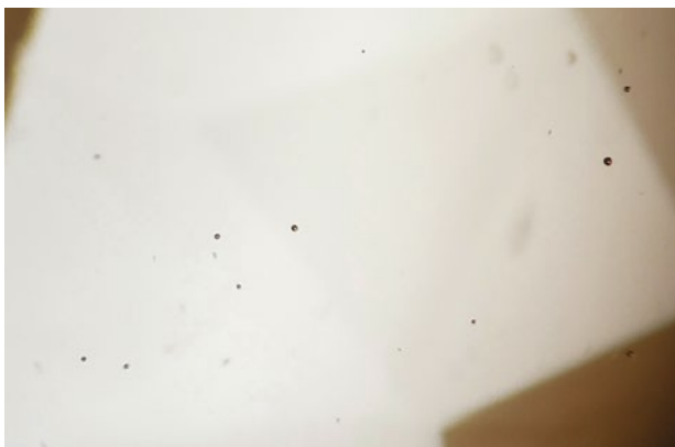
Figure 40: Tiny, round gas bubbles such as these were present in all of the glass imitations of tanzanite. Photomicrograph by B. Williams; image width 5.2 mm.
