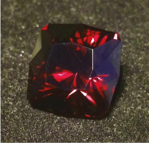
Figure 37: One of three faceted specimens cut from the boule fragment in Figure 36 is this 35 ct (1.85 cm across) synthetic tephroite. The colour is due to the presence of Mn in the tephroite structure. Photo by J. Rakovan.
