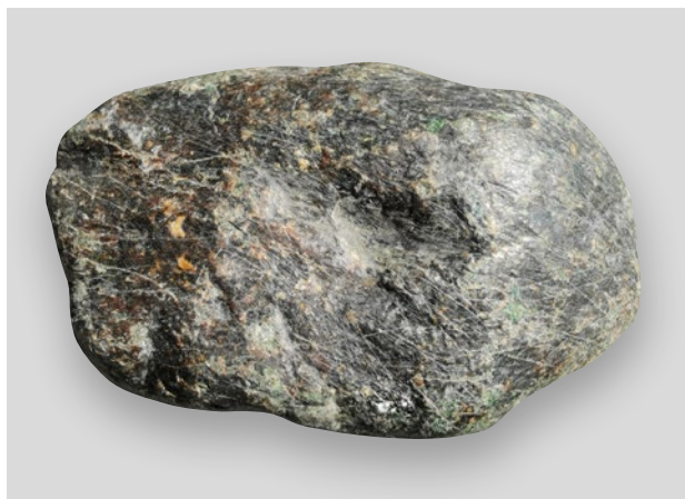
Figure 42: The 'crust' of this 631.68 g jadeite sample was identified as consisting of an artificial green powdery layer overlain by a brown mixture of wax and epoxy. Photo by W. Lu.
