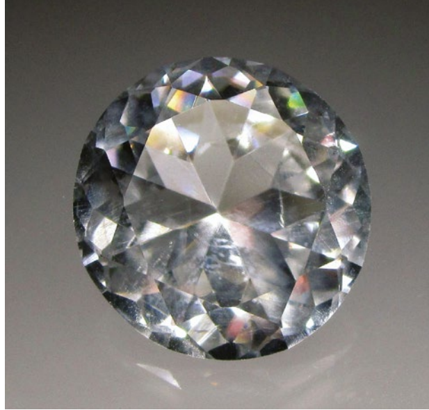
Figure 38: This 30 ct (2.1 cm diameter) synthetic forsterite is one of five faceted samples cut from a colourless boule. Colourless forsterite is extremely rare in nature because Fe is usually present to impart green colouration. Photo by J. Rakovan.
