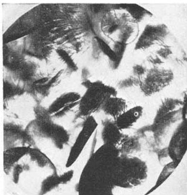
FIG. 2.—Leaf-like stress figures artificially induced in amber.
