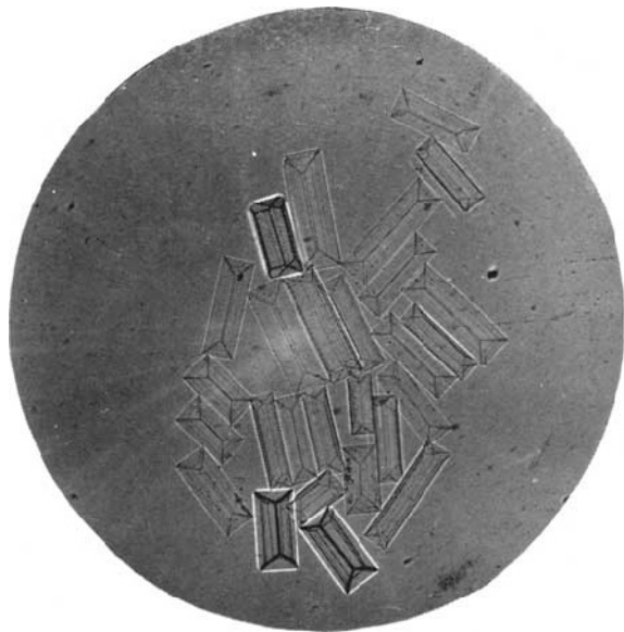
Fig. 3. Enlarged immersion contact photograph of synthetic corundum (faint outlines), and synthetic spinels (three stones with bolder outlines) immersed in methylene iodide. "Line" film used, 3 seconds exposure.
