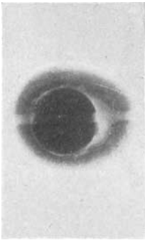
Fig. 4. Radiograph of a drop-shaped cultured pearl showing an excess of conchiolin at one end thus producing the pear shape, the bead nucleus being spherical.
