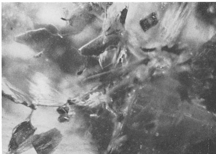
Fig. 10. Individual flakes of biotite. 80 ×.
