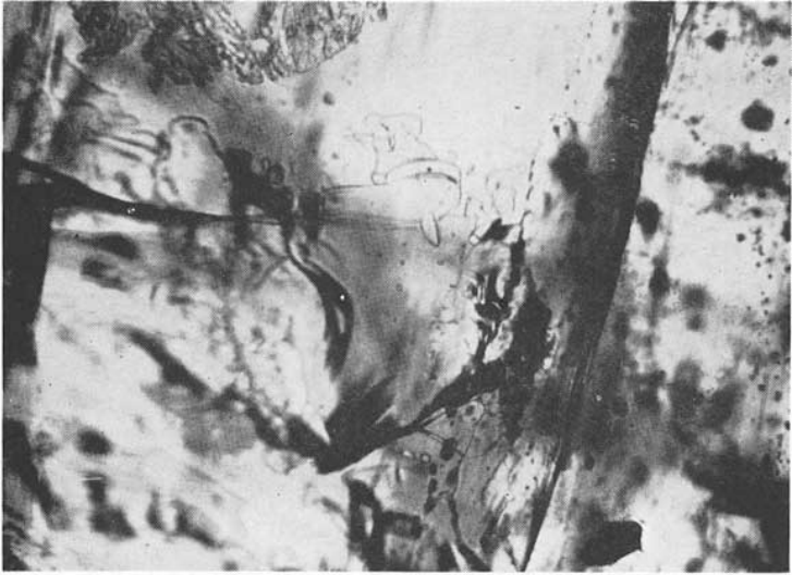
Fig. 7. Liquid and solid inclusions. 75 ×.
