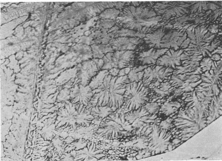
Fig. 19. Solar pattern of re-crystallization centres in healed fissures in Burma sapphire. 75 \times .
