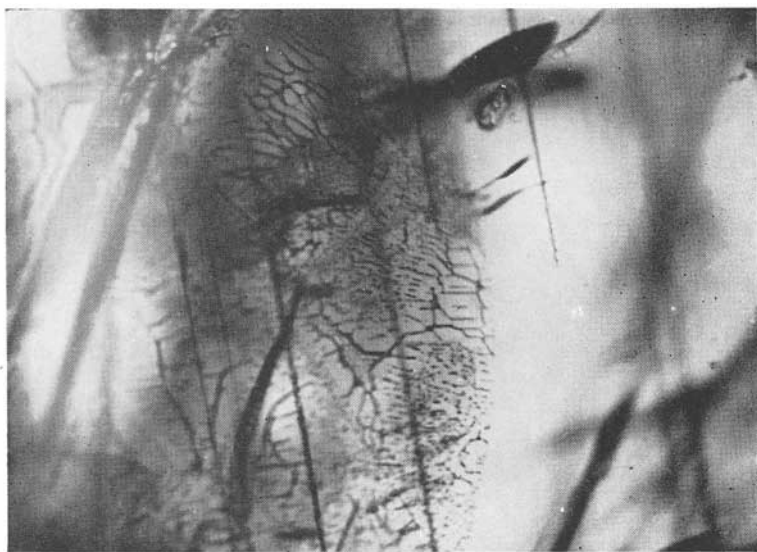
Fig. 21. Network of residual liquid drops of a healed fissure traversing several twin lamellae in Siam ruby. 75 \times .
