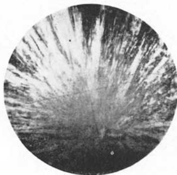
Synthetic moonstone-coloured spinel possessing chatoyancy. 32x. Structure picture between crossed nicols.
