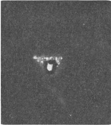
Fig. 10. So-called "bubble" in a German synthetic star-stone seen as a two-phase inclusion.
