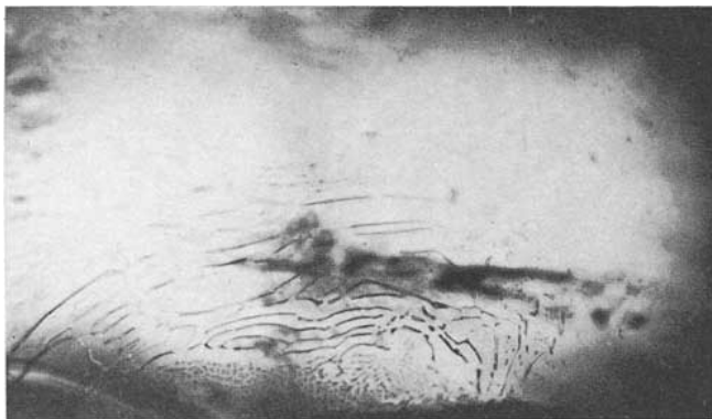
FIG. 13. Alum crystal. A healing crack emanates from the growth disturbance. The healing crack developed during growth of the crystal, but is not oriented. It can be compared with secondary healing cracks in many precious stones. 50 ×
