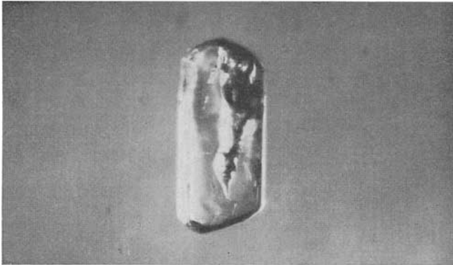
FIG. 11. Chatham's synthetic emerald. Inclusion of phenakite crystal of prismatic shape. 120 ×
