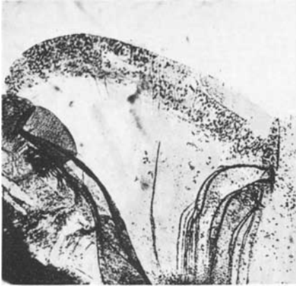
FIG. 17. Cleavage crack parallel to the Octahedral plane of a diamond. 110 ×
