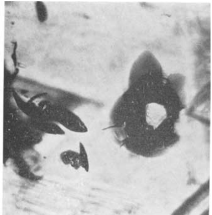
FIG. 6. Olivine inclusion encircled by strongly developed cleavage cracks. 65 ×
