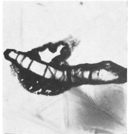
FIG. 12. Apatite inclusion in diamond showing cleavage cracks. 220 ×
