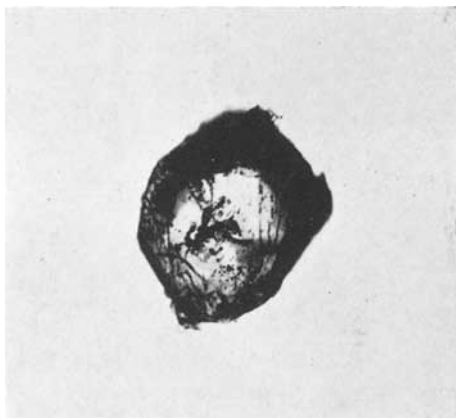
FIG. 7. Olivine inclusion after separation (see Fig. 6) containing inclusions of an unknown nature. 120 ×
