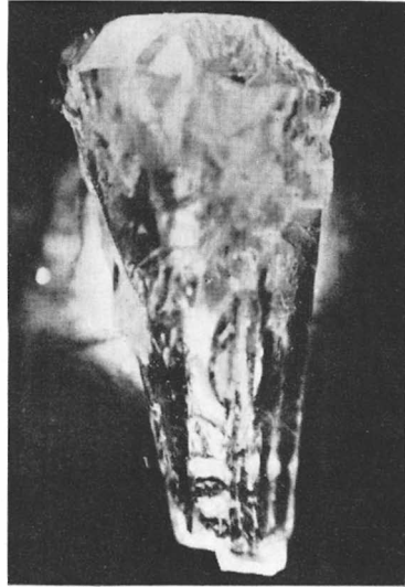
FIG. 15. Three-phase inclusion in a Chivor emerald. To the left of the black round gas bubble is the square outline of a halite crystal. Notice the elongated outline of the inclusion cavity. These inclusions are part of a healing fissure. Usually the bubble in a Colombian three-phase inclusion is stationary. Recently a moveable bubble has been found.
