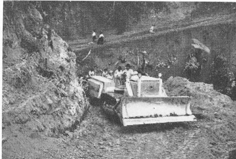
FIG. 12. Bulldozer pulling an air compressor and making its own road through Cretaceous shale on the way to the mine. The bulldozer is used during the mining operation to remove the overburden.
