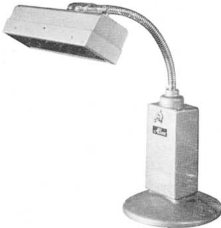
An English long-wave ultra-violet lamp, the ALLEN lamp, is a fluorescent tube lamp with twin tubes and has a separate filter attached to the removable cover.
