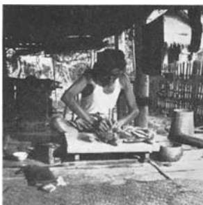
FIG. 1. Jade lapidary squatting behind his low bench is polishing small cabochons and buttons.
