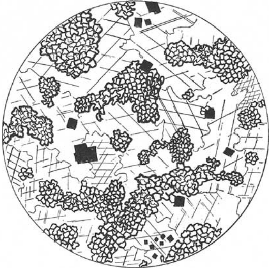
FIG. 2. Normal blue Siberian lapis-lazuli. The fine grained lazurite is set in coarse grained calcite and a few opaque cubes of pyrite are also visible. Diameter of field approx. 1.8 m.m.
