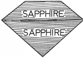
Schematic diagram of a true doublet.
