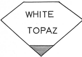
An unusual type of doublet. The stone is white or very pale pink topaz and the tip of the pavilion is made of natural blue sapphire. The effect was not very good, and the expected total blue coloration of the stone by total internal reflection did not occur.
