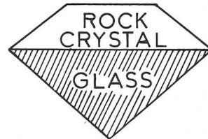
Schematic diagram of a false doublet.
