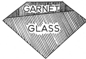
Schematic diagram of a garnet-topped doublet.
