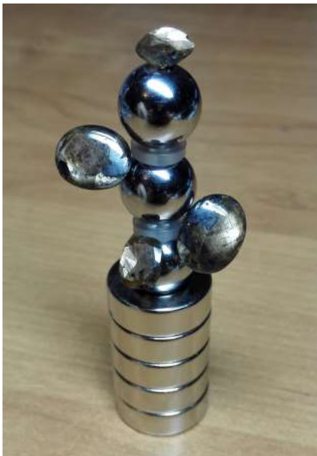
Figure DD-8: This stack of five disks and three spheres of neodymium-iron-boron magnets, with a maximum energy product of 42 MGOe, attracts four samples of gold-sheen sapphire that contain large surface-reaching inclusions of magnetite. The two faceted stones (top and bottom) weigh 1.56 and 2.91 ct, and the two cabochons weigh 5.52 and 8.84 ct. The magnetite is easily visible in the two cabochons as silvery grey areas. Photo by T. N. Bui.
