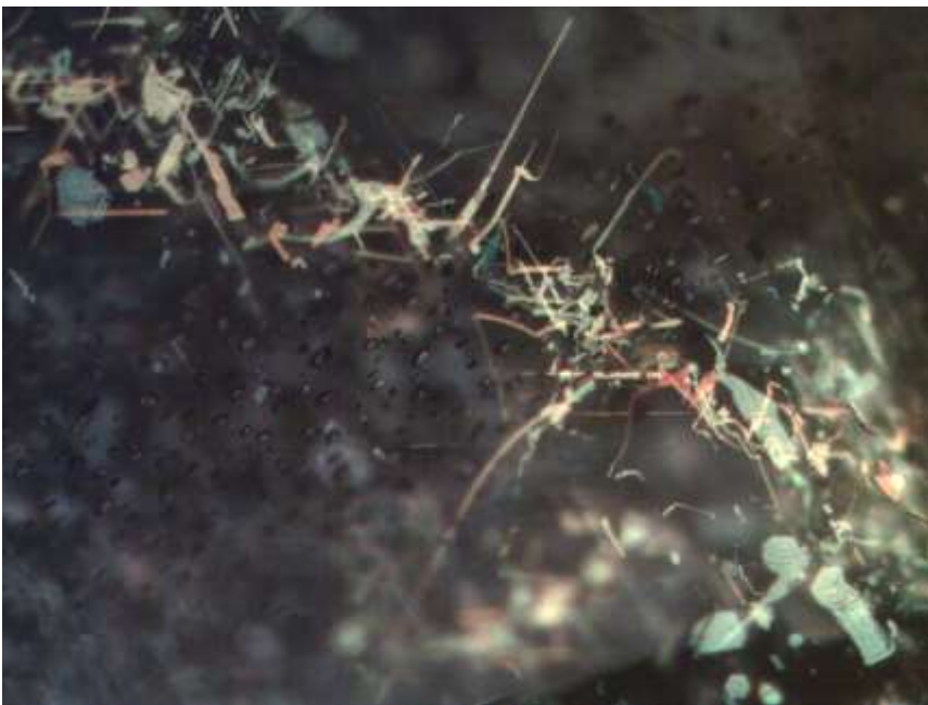
Figure DD-4: Needles/platelets and negative crystals are shown in this image of a gold-sheen sapphire. Photomicrograph by T. N. Bui using brightfield illumination; magnified 50x, field of view 1.0 x 1.3 mm.
