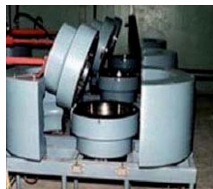
Figure B9: View into a production hall with BARS type presses in Novosibirsk, Russia; the equipment is used for diamond synthesis and diamond treatments. Photograph by courtesy V. Vins, Institute of Single Crystals, Novosibirsk, Russia.
