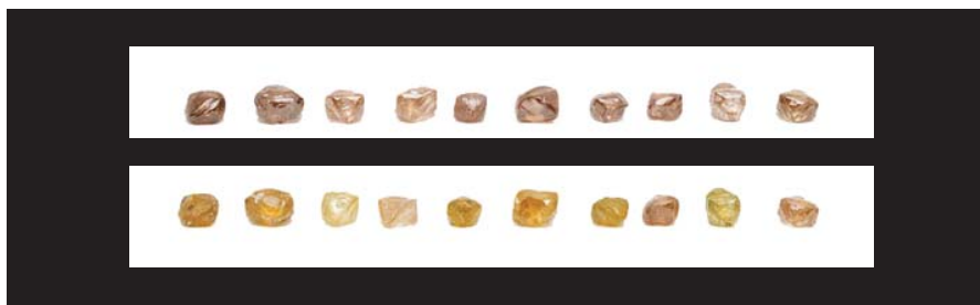
Figure 11: Suite of originally brown to yellowish brown diamonds before (above) and after HPHT treatment; weights range from 0.75 to 0.95 ct. Photograph by courtesy of J.-P. Chalain, SSEF Swiss Gemmological Institute, Basel, Switzerland.
