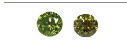
Figure 4: These type Ia diamonds of 1.20 ct (left) and 1.10 ct were originally brown and treated in a HPHT process. Photograph courtesy of E. Erel, Carat Gem Lab, Gemological Laboratory, Montigny-les-Metz, France.
