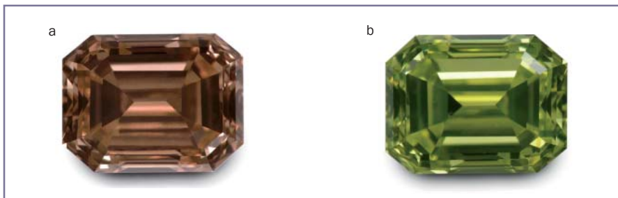
Figure 14 a,b: This type Ia diamond of 2.10 ct (a) was originally brown and treated in a HPHT process and became yellowish green (b). Photograph by courtesy of T. Hainschwang, Gemlab, Gemmological Laboratory, Balzers, Liechtenstein.
