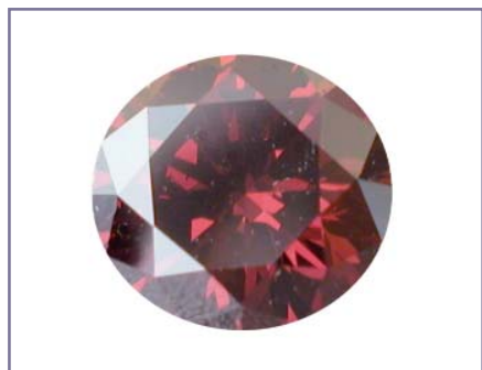
Figure 5: This type Ia diamond of 1.51 ct was originally brown and treated in a three-step process by a) HPHT, b) electron irradiation and c) annealing. Photograph by courtesy of V. Vins, Institute of Single Crystals, Novosibirsk, Russia.
