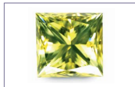
Figure 6: This type Ib synthetic diamond of 0.33ct was originally intense yellow and treated in a HPHT process. Photograph by courtesy of T. Hainschwang, Gemlab, Gemological Laboratory, Balzers, Liechtenstein.
