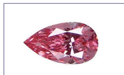
Figure 9: This type IIa diamond of 0.50 ct was originally brown and treated in a HPHT process. Photograph by courtesy of E. Erel, Carat Gem Lab, Gemological Laboratory, Montigny-les-Metz, France.
