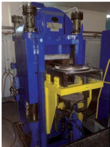
Modified Bridgman-type HPHT apparatus
