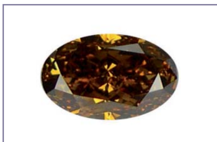
Figure 13: This type Ia diamond of 1.30 ct was originally brown and treated in a HPHT process. Photograph by courtesy of E. Erel, Carat Gem Lab, Gemmological Laboratory, Montigny-les-Metz, France.
