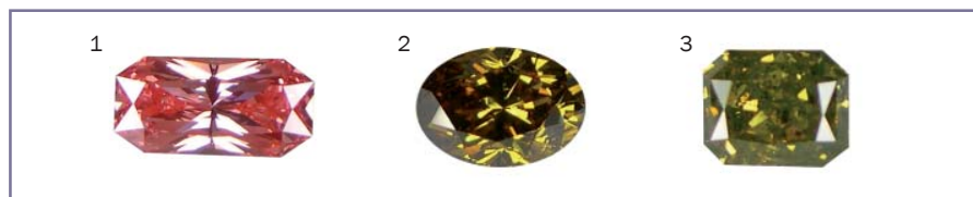
Figure 1: This type IIa diamond of 1.20 ct was originally brown and treated in a HPHT process. Figures 2 and 3: These type Ia diamonds of 1.00 ct and 1.60 ct respectively, were originally brown and treated in a HPHT process. Photographs courtesy of E. Erel, Carat Gem Lab, Gemological Laboratory, Montigny-les-Metz, France.
