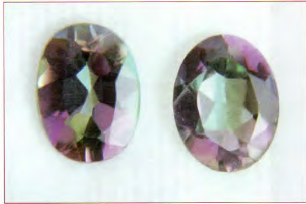
Figure 2: These two 'fire topazes' are surface-coated with thin metallic layers deposited on the pavilion or the crown facets. Such stones may appear under different trade names. Various optical reflection, transmission and interference phenomena cause different coloration (from green to violet) when the samples are viewed at different angles. The stones are 9.2 × 7.0 mm, weights 2.27 and 2.21 ct. Photo by M. Glas.
