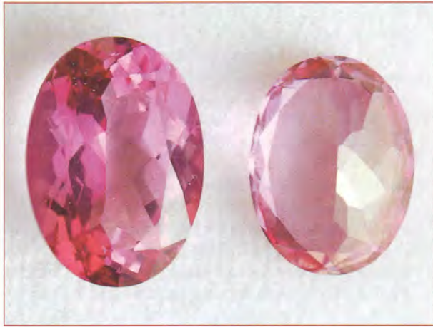
Figure 5: These two pink topazes are dye-coated on the pavilion facets of the samples. Different colour intensities are observed when viewed through the colourless crown and through the dyed pavilion. The stones are 18.0 × 13.0 mm and 15.8 × 12.0 mm, weights 15.17 and 10.59 ct. Photo by M. Glas.
