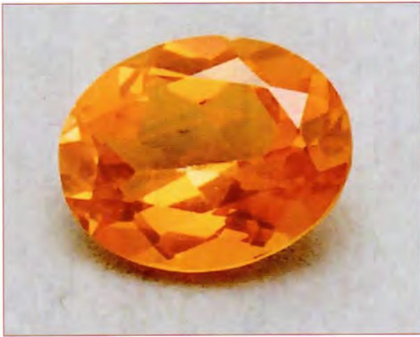
Figure 1: This surface-coated topaz is coloured by a thin iron-bearing layer on the pavilion of the stone; similar stones have been offered to gem dealers in Nigeria as natural topaz. The stone measures 10.1 × 8.0 mm, weight 2.95 ct. Photo by M. Krzemnicki, SSEF, Basel.
