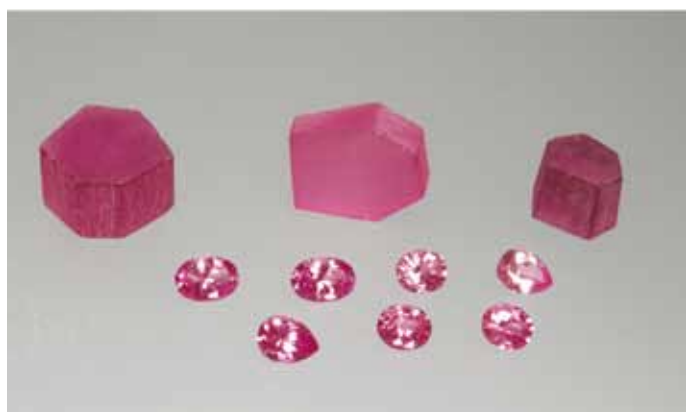
Figure 2: Rough and faceted titanium-bearing synthetic chrysoberyls produced by Kyocera in Japan in daylight (above) and incandescent light; size of the rough crystal above left 16.0 x 15.5 x 10.0 mm, weight 34.12 ct, the faceted sample below left weighs 1.08 ct and measures 7.8 x 5.7 mm. Photo by K. Schmetzer.
