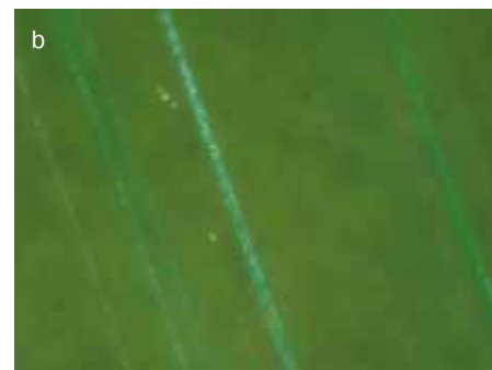
Figure 16a,b: Thin sections of Kyocera chatoyant synthetic alexandrites oriented almost perpendicular to the b pinacoid show layers parallel to the a plane with numerous tiny needles alternating with layers of transparent alexandrite. The layers are thicker in b . Reflected light, crossed polarizers, field of view 112 x 84 \mu\text{m} . Photos by H.-J. Bernhardt.
