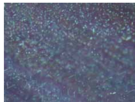
Figure 15: A thin section of a star synthetic alexandrite from Kyocera oriented almost parallel to the a pinacoid shows three series of needles which form angles near 60^\circ to each other. Reflected light, crossed polarizers, field of view 112 x 84 \mu\text{m} . Photo by H.-J. Bernhardt.
