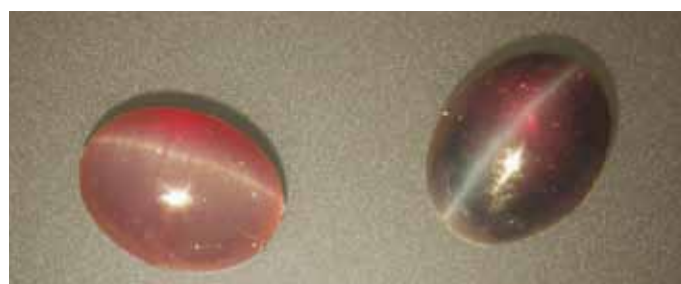
Figure 4: Synthetic alexandrite cat's-eyes produced by Kyocera in Japan in daylight (above) and incandescent light; sample C2 with lower Ti^{3+} contents weighs 3.29 ct and measures 9.2 x 7.2 mm, sample C3 with higher Ti^{3+} contents weighs 3.19 ct and measures 9.2 x 7.1 mm. Bosshart collection. Photo by K. Schmetzer.
