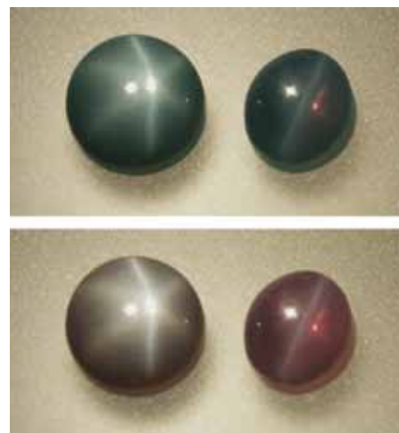
Figure 1: Synthetic asteriated alexandrite (left, 2.62 ct, diameter 8.0 mm) and synthetic alexandrite cat's-eye (1.55 ct, 7.0 x 6.0 mm) produced by Kyocera in Japan in daylight (above) and incandescent light. Photo by K. Schmetzer.
