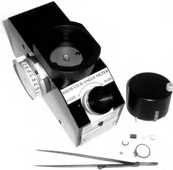
Figure 9.30 View of a gemstone on the test platform. The laser beam can only be activated when the circular test platform cap is in position and the knurled test button on the right of the cap is pressed
