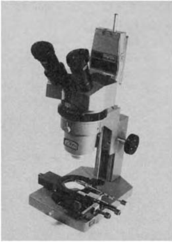
Figure 9.23 A Krüss microscope fitted (at top rear) with an electronic gauge for RI measurement by the 'direct' method
