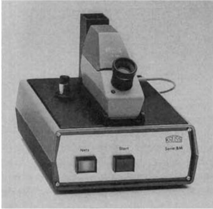
Figure 9.15 The Krüss high-range refractometer used a strontium titanate prism and a heated thermoplastic paste as a contact fluid. Because of the high dispersion of strontium titanate the refractometer's control plinth contained a sodium light source
