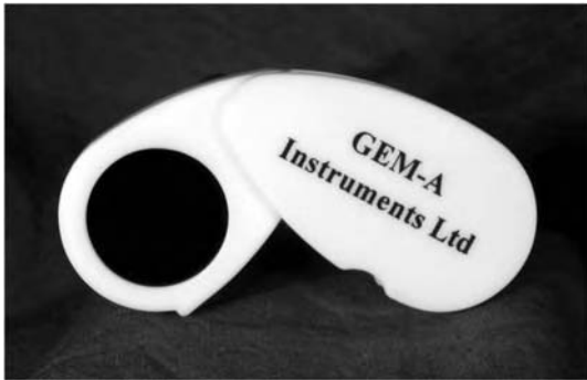
Figure 13.15 The Chelsea filter transmits light in the red and green wavelengths to match emerald's red transmission and yellow-green absorption. (Gem-A Instruments Ltd)
