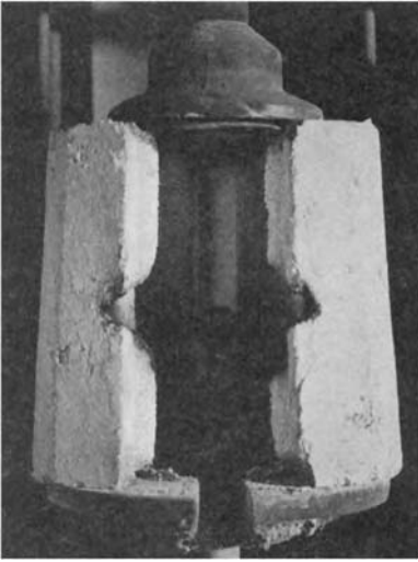
Figure 15.2 Interior of a Verneuil furnace showing the finished boule. (D. Swarovsky)
