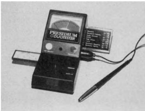
Figure 12.12 The 'Duotester' is a combined reflectance meter and thermal conductance tester. The slide drawer on the left contains a range of diamond simulants for use when checking calibration. The pull-out panel on the right lists typical reflectance readings which appear on an LED display in the front edge of the instrument
