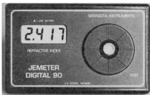
Figure 9.17 The 'Jemeter Digital 90' reflectance instrument measures gemstone RIs to three decimal figures over the range 1.450–2.999. Fitted with a polarizing filter, it can also detect double refraction down to 0.01
