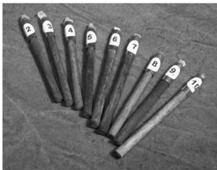
Figure 6.1 A set of nine hardness pencils from a boxed set. (Gem-A Instruments Ltd)
