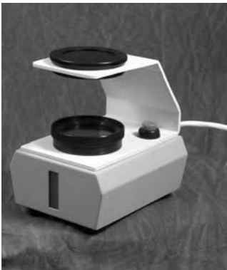
Figure 10.4 A typical table polariscope (the small light port on the lower front can be used as a refractometer light source). (Gem-A Instruments Ltd)
