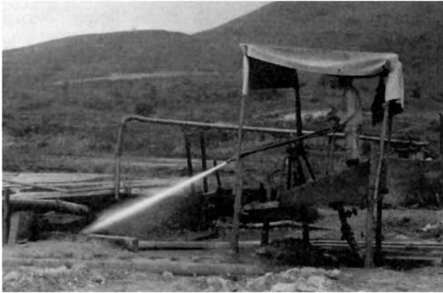
Figure 2.11 Using a high-pressure water jet to separate topaz crystals from a mixture of mineralized clay and kaolin at the Capo do Lana mine in Brazil
