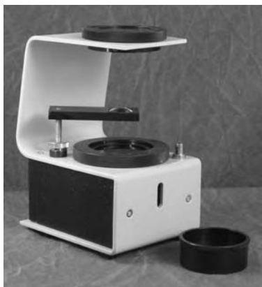
Figure 10.7 A polariscope fitted with a conoscope lens and supplied with an immersion dish. With the lens pivoted between the two filters the instrument can be used to view interference figures. (Gem-A Instruments Ltd)
