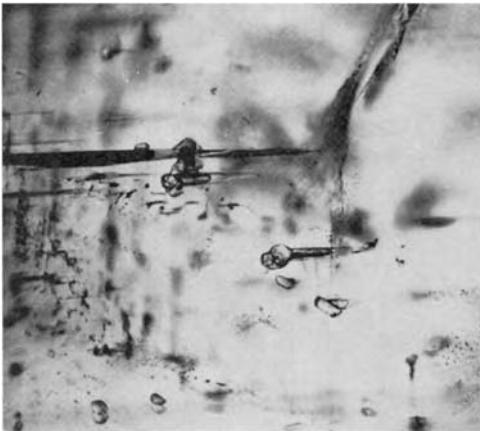
Figure 16.10 Nail-like inclusions formed by a phenakite crystal capping a needle/conical tube in a Linde hydrothermal synthetic emerald
