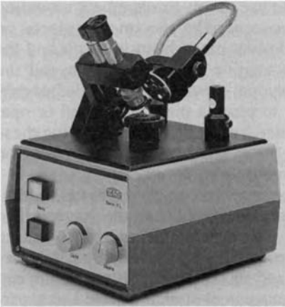
Figure 11.7 A prism spectroscope unit with built-in fibre-optic illumination. The disc at the end of the light guide is fitted with colour filters to improve the contrast of spectra. The light port at the rear right-hand side is for refractometer illumination
