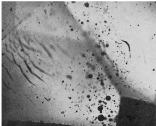
Figure 16.16 Fire marks (surface cracks caused by over-pressure polishing) and bubbles in a synthetic ruby
