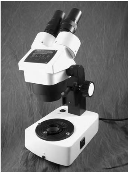
Figure 13.10 A typical stereo zoom microscope with overhead and light/dark-field illumination and a magnification of 0.7–45 \times using 10 \times eyepieces, a range which can be doubled with 20 \times eyepieces. (Gem-A Instruments Ltd)
