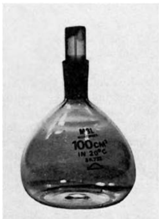
Figure 7.2 An SG bottle (also called a pycnometer) can be used to measure a small gemstone's SG by the displacement method. It is designed, however, for the precise determination of the SG of liquids (see end of chapter)
