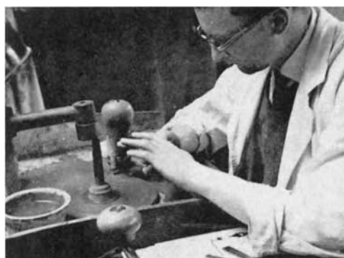
Figure 19.18 (top left) The bow-driven vertical polishing lap still used by some native lapidaries in India and Sri Lanka. (above) Sketch showing the use of the jamb peg. (left) A lapidary using a jamb peg (on the far side of the lap)
