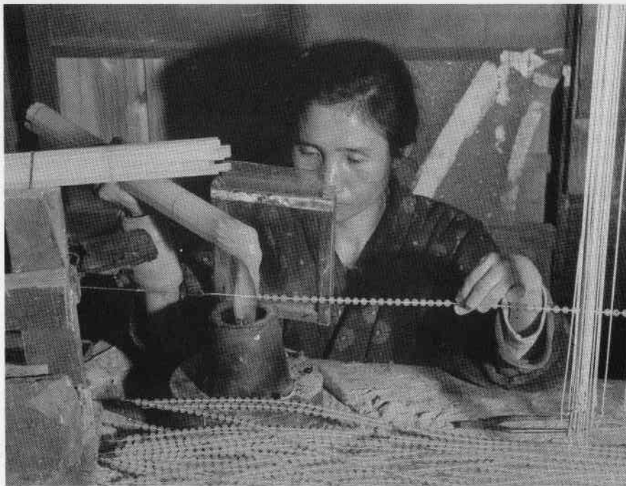
Making glass beads for imitation pearls. The wire suspended over a kerosene burner rotates slowly and drops of molten glass from the rod, held by the artisan, fall on the wire and form glass beads
