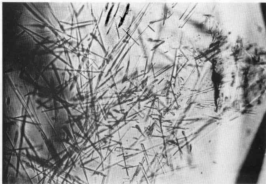
Figure 4. Remarkably short tremolite rods being a typical feature of Sandawana emeralds. 125x
