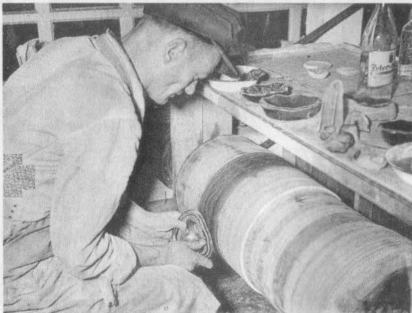
Polishing an agate ashtray on a large felt-covered wooden drum. Turned by water power.
