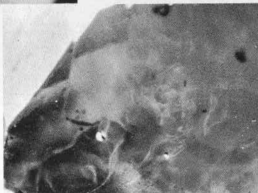
Inclusions of metallic crystals in synthetic emeralds.
