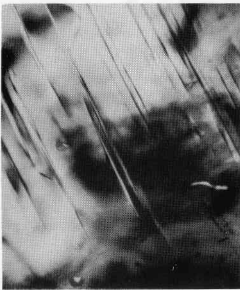
Figure 5 System of parallel lines form the traces of polysynthetic lamellae.
