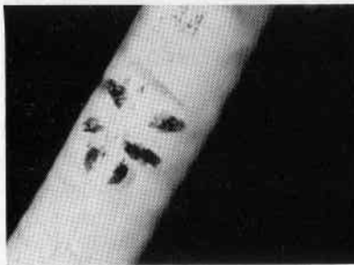
Figure 17. If the specimen is tilted into an appropriate position, an interesting mirror effect of natural inclusions in the beryl nucleus is brought about by the artificial emerald layer. (Diamondscope. 40x)
