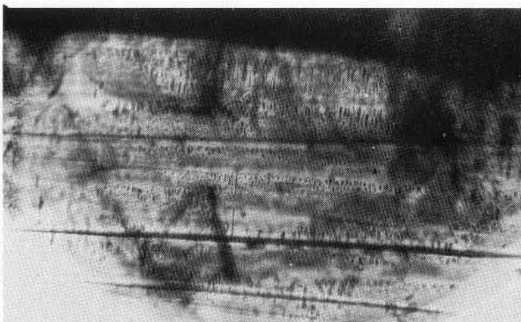
Figure 2 Banded lateral appearance caused by horizontal fluid ribbons and zonal structure (75x).
