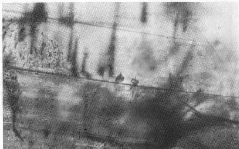
Figure 5 Minute seed crystals of phenakite, formed on the surface of the last layer when alumina concentration was low. Tiny growth funnels had just started to grow on the microlites.
