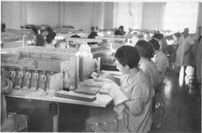
The larger beads are individually set in short lengths of wire to make up pincushion-like rectangles
