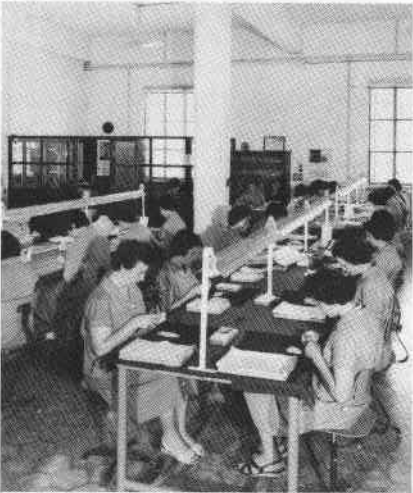
Nipping off the hanging drop of excess essence coating, the final preparation step
