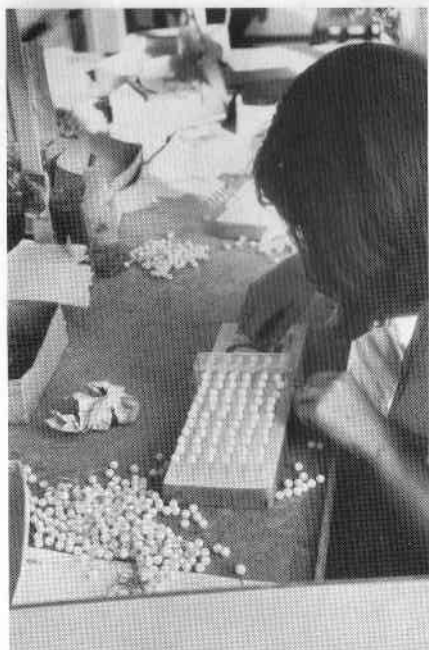
Individually mounted beads on wires are set into blocks that are inverted into the lacquer-filled trays
