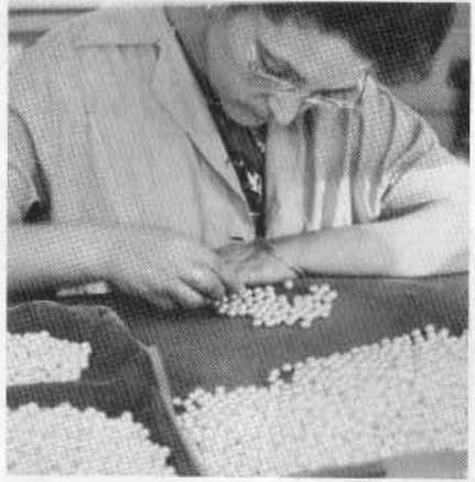
Checking the finished pearls for any blemishes that would make them unacceptable for the finest strands
